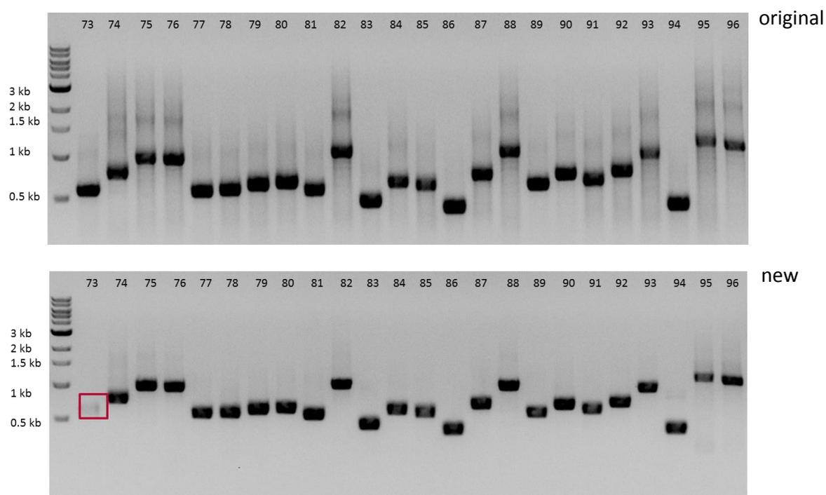
**Figure 15: Plackett-Burman test set for SPCR: Here an excerpt of the 96 sequence analysis data is shown (sample 73 – 96); marked in a red box is one sequence that failed after shortening the protocol for the thermo cycler; 7 µl of 1kb ökladder from NEB were used as a reference.**
