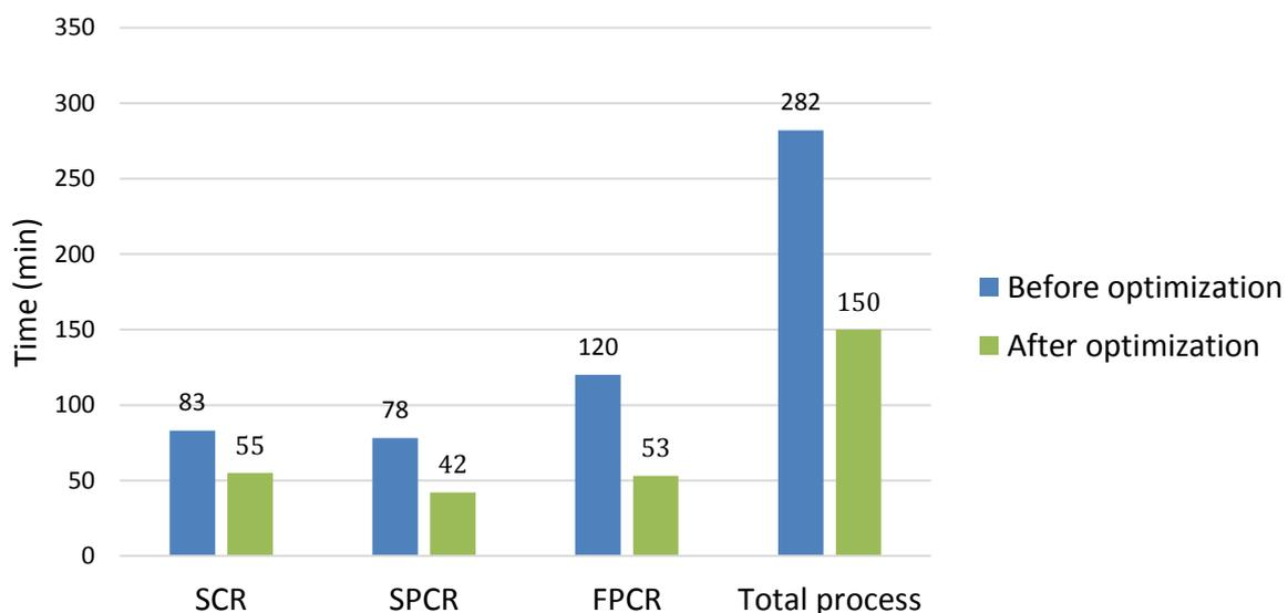
**Figure 37: Turnaround time in comparison: overview on SCR, SPCR, FPCR and the total process; the blue bars represent the initial times and the green bars the times after PBD optimization; time is given in minutes.**
