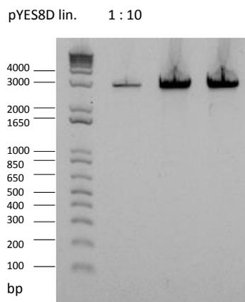
**Figure 32: Linearization pYES8D by PCR: 5  $\mu$ l of 1 kb Plus ladder were used as a reference; On the 1% E-Gel 1  $\mu$ l of the PCR reaction was loaded together with a 1 : 10 dilution; all samples show distinct bands in the expected size of 2848 bp.**
