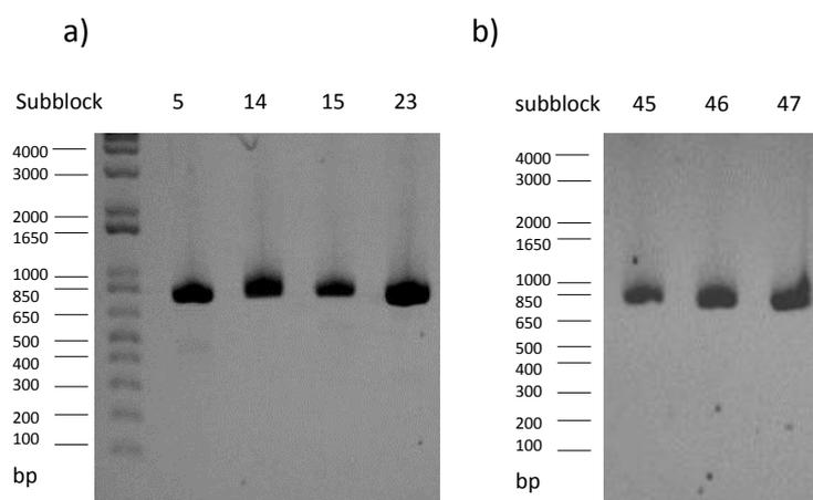
**Figure 21: Amplification of subblocks:** 5  $\mu$ l of 1kb Plus ladder were used; a) Subblocks 5 (854 bp), 14 (847 bp), 15 (854 bp) and 23 (847 bp) have an internal XhoI restriction site and were thus amplified by PCR from the ordered plasmid; b) Subblocks 45, 46 and 47 (854 bp each) were also amplified by PCR due to a failed restriction digest; shown here all samples were loaded on a 1% E-Gel and documented.
