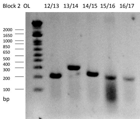
**Figure 30:** *E. coli* colony PCRs from the assembled blocks: 1  $\mu$ l of each PCR reaction was loaded on a 2% E-Gel; amplification products are the overlapping regions (OL) between the assembled subblocks; all connecting regions are amplified and distinct visible bands appeared in the expected sizes of 174 bp, 247 bp, 207 bp, 187 bp, 174 bp; 5  $\mu$ l of 1 kb Plus ladder were used as a reference.
