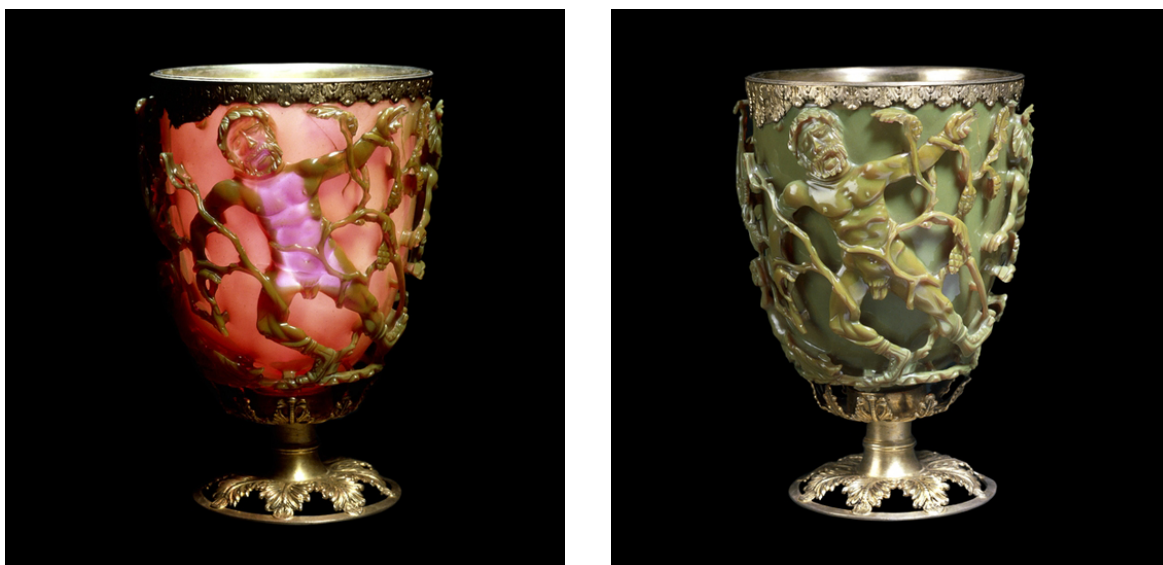
Figure 15: The Lycurgus cup. Ancient artifact from the late Roman period (approx. 4th century AD) in the British Museum. Fine gold and silver nanoparticles incorporated in the glassware create different color impressions for transmitted (left) and reflected (right) light due to surface plasmon resonance. Licensed under Creative Commons, reprinted from reference [173].
