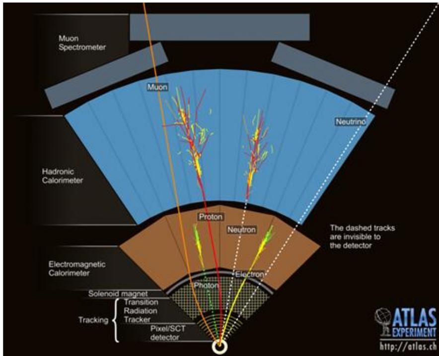
Figure 3.3.2.: ATLAS detector with particle tracks and showers. Image from Ref. [30].
