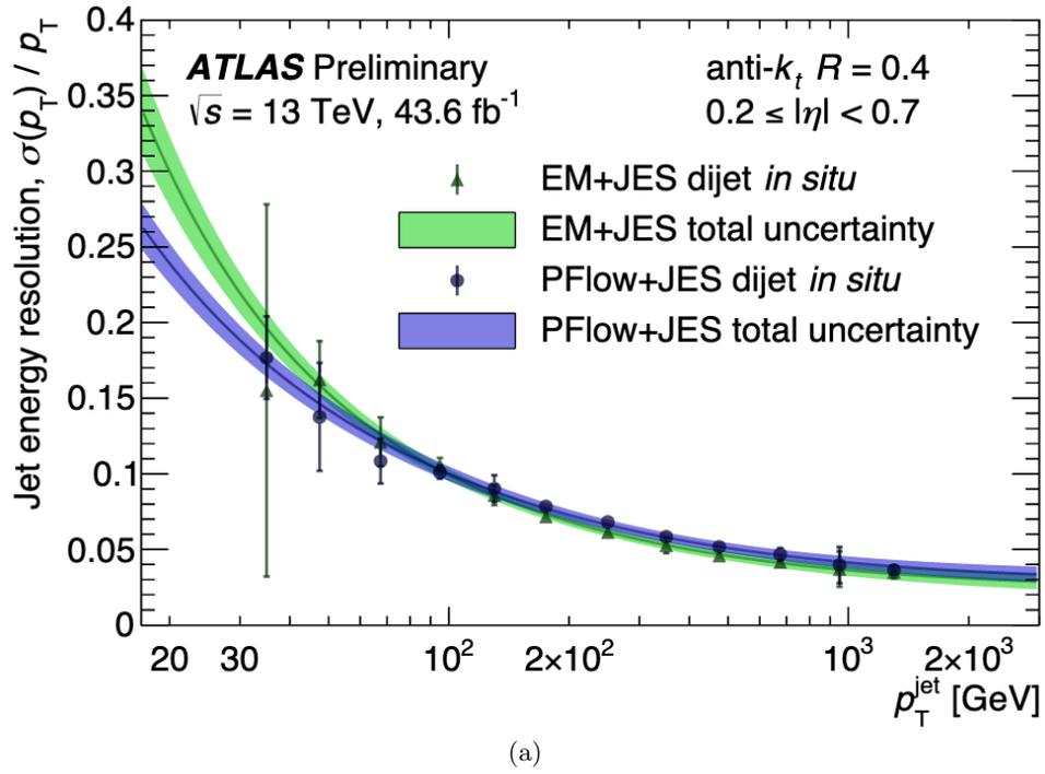
Figure 5.4.10.: Jet energy resolution as a function of jet  $p_T$ . Image from Ref. [87].
