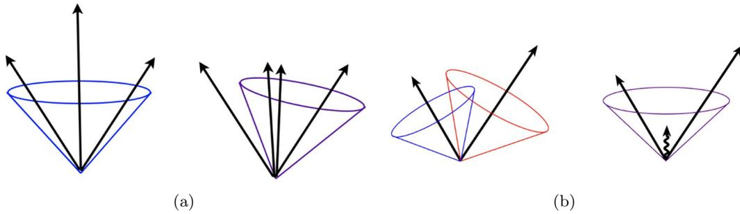
Figure 5.4.2.: (a) Example of collinear unsafety. The jet is changed due to a collinear splitting. (b) Example of infrared unsafety. Jets are merged after the emission of a soft particle [79].
