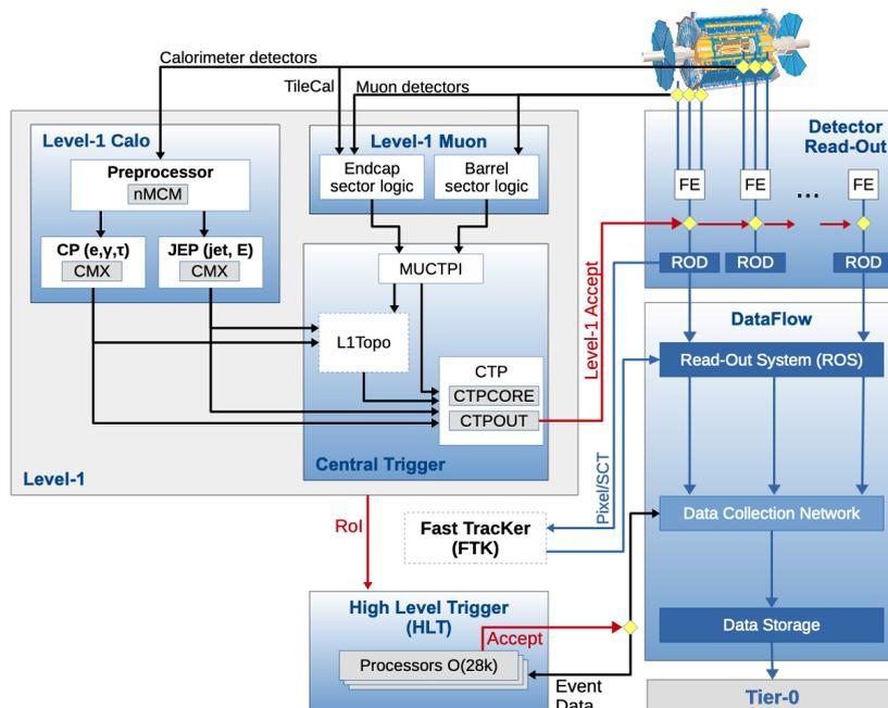
Figure 3.4.1.: Schematic overview of the ATLAS trigger and data acquisition system in Run 2. Image from Ref. [43].
