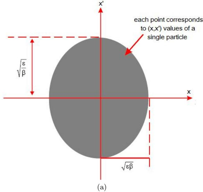
Figure 3.2.1.: The emittance is the area (length  $x \times$  angle  $x'$ ) of the ellipse [26].
