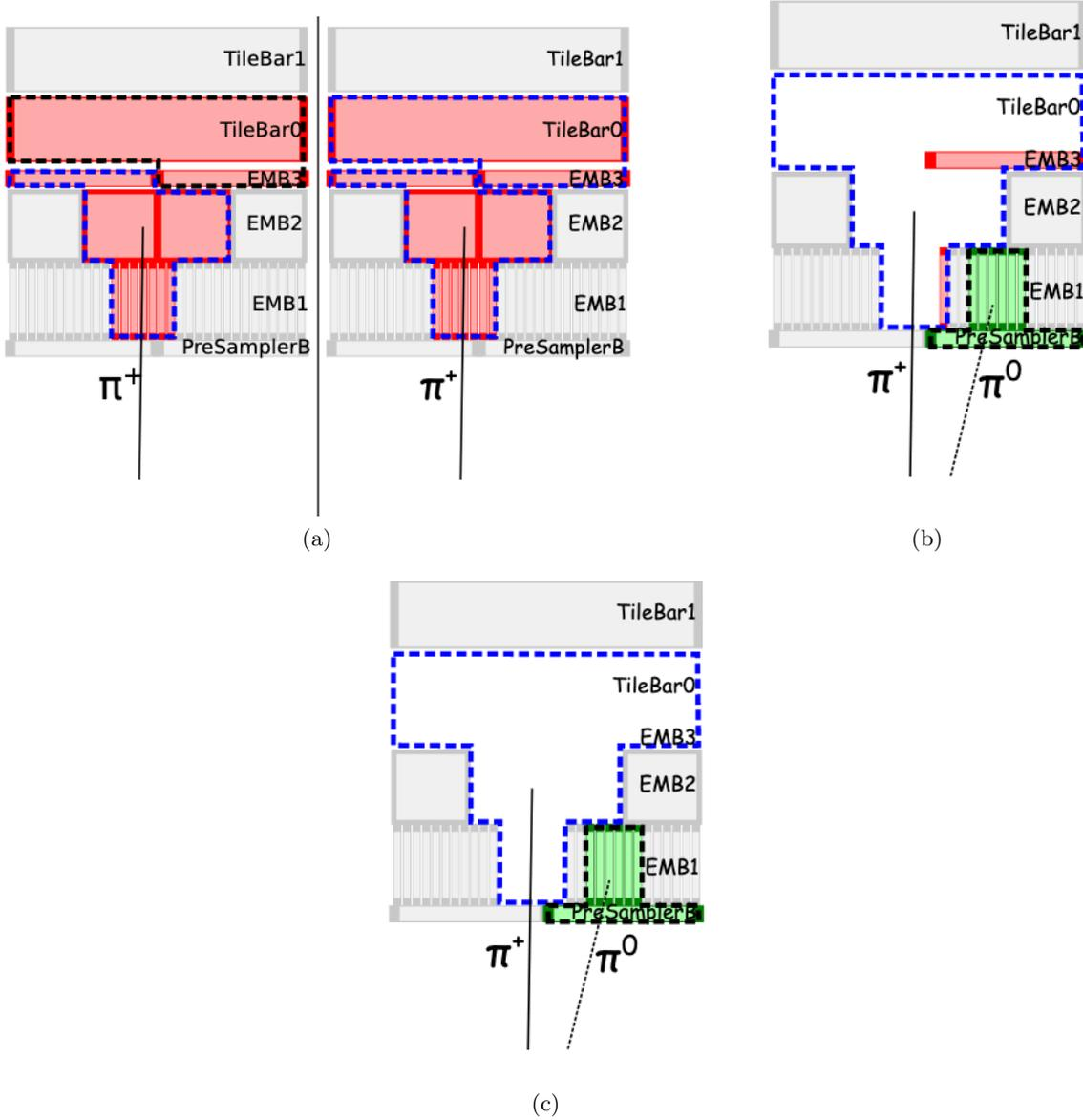
Figure 5.4.6.: The shower subtraction procedure in PFlow algorithm dealing with different cases as discussed in the text. The red cells associated to tracks represent charged hadrons, while green cells without a track close by are recognized as a neutral hadron or the photons. The dotted line means the boundaries of the selected cells by the algorithm. Three electromagnetic calorimeter layers and two tile calorimeter layers are shown. Image from Ref. [83].
