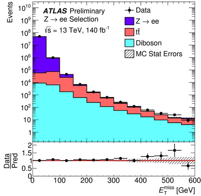
Figure 5.6.10.: Modelling of PFlow  $E_T^{\text{miss}}$ . The  $Z \rightarrow ee$  sample is produced with POWHEG. Diboson samples include:  $WW \rightarrow \nu\nu\nu$ ,  $WZ \rightarrow \nu ll$ , and  $ZZ \rightarrow \ell\nu\nu$ . Image from: Ref. [103].
