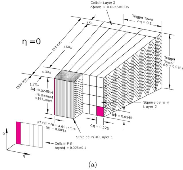
Figure 3.3.6.: A view of the EMCAL module located at  $\eta = 0$  in the barrel. Image from Ref. [33].
