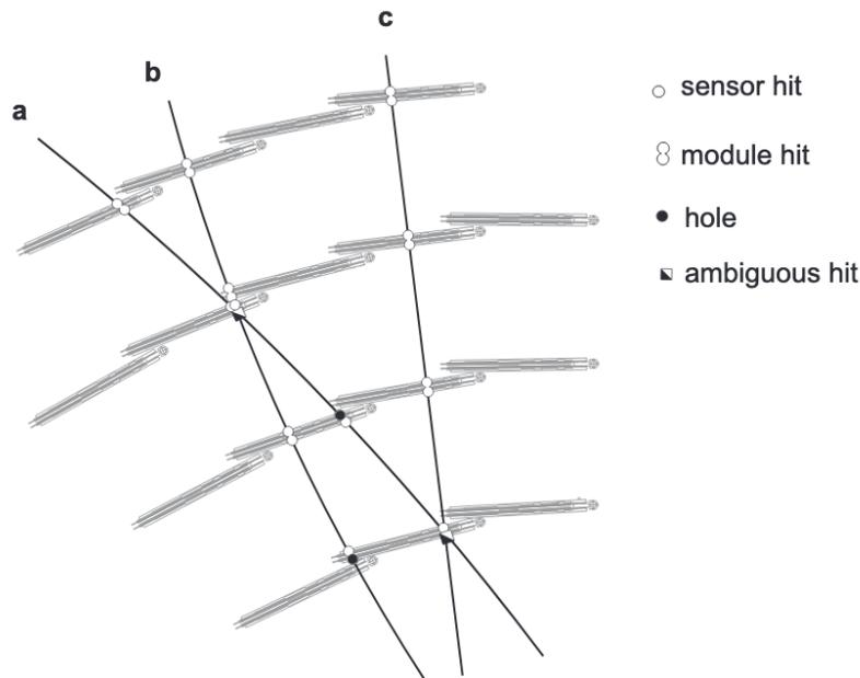
Figure 5.1.1.: Inside-out track reconstruction in the SCT: seeding and track finding with ambiguity solving. Image from Ref. [69].
