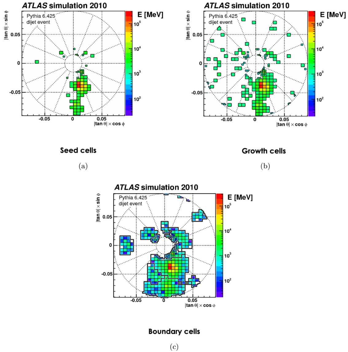
Figure 5.4.3.: Building a 4-2-0 topo-cluster. Figure (a) shows the individual calorimeter cells that are chosen if cells have  $\xi > 4$ . Figure (b) shows the adjacent cells to the seed when  $\xi > 2$  are added. Figure (c) shows the tertiary cells with  $\xi > 0$  [80].
