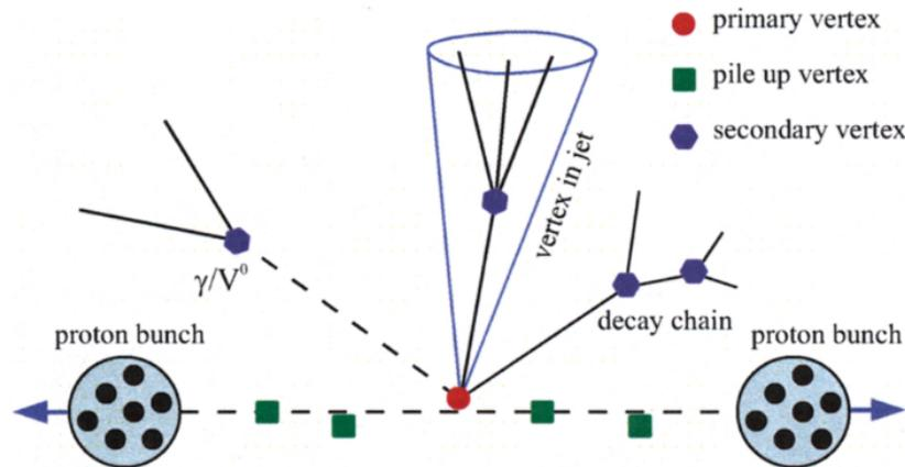
Figure 5.1.3.: The topologies of primary vertex, pile-up vertex and secondary vertex. Image from Ref. [72].
