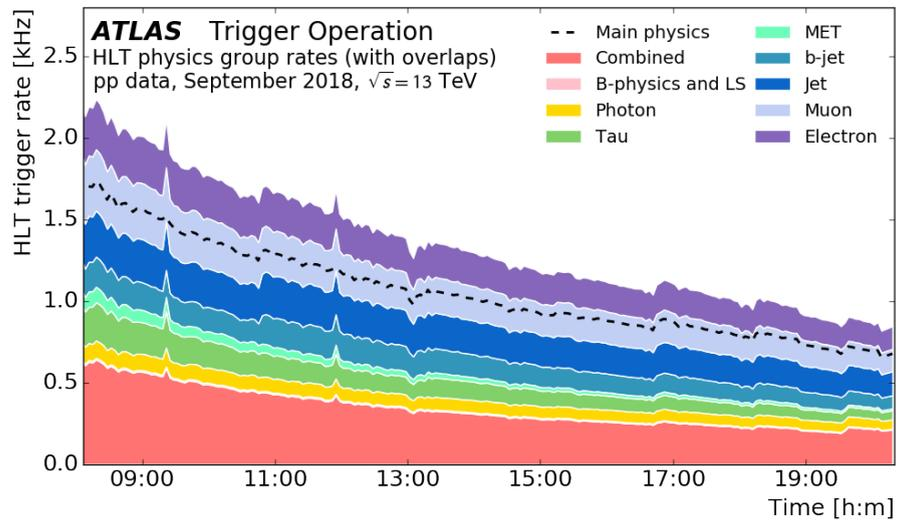
Figure 3.4.2.: HLT physics trigger group rates as a function of time in a fill taken in 2018 [45].
