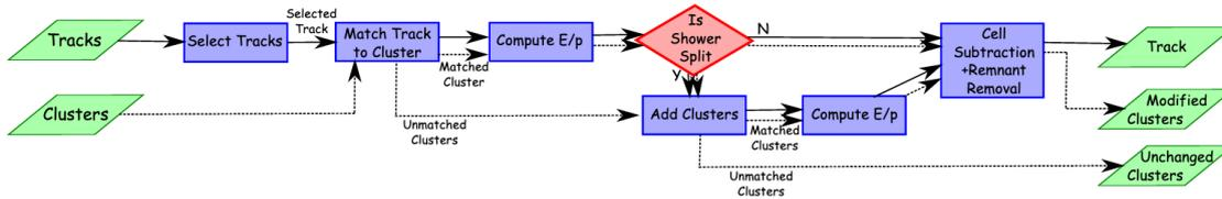
Figure 5.4.5.: A flow chart shows how the neutral particle flow (nPFOs) and charge particle flow (cPFOs) objects proceed. Image from Ref. [83].
