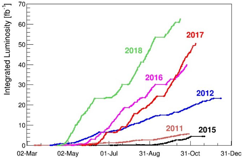
Figure 3.2.2.: Integrated luminosity delivered by the LHC machine to the ATLAS and CMS detectors experiments during the 2011 to 2018 runs [27].
