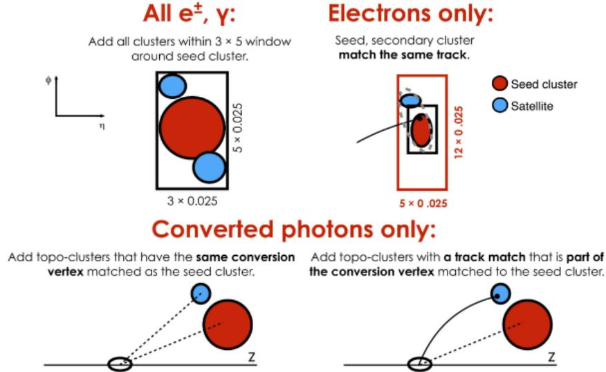
Figure 5.2.1.: Diagram of the super-clustering algorithm for electrons and photons. Seed clusters are shown in red. Satellite clusters in blue. Image from Ref. [73].
