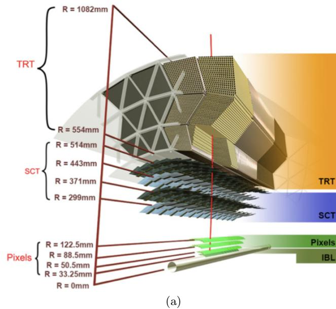
Figure 3.3.3.: The beam pipe, the IBL, three Pixel layers, four cylindrical layers of the SCT and the TRT are shown for the ID in the barrel region. Image from Ref. [33].
