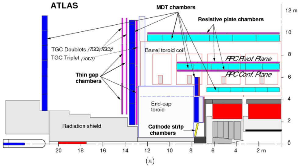
Figure 3.3.7.: A schematic representation of the muon spectrometer in the z-y projections [41].
