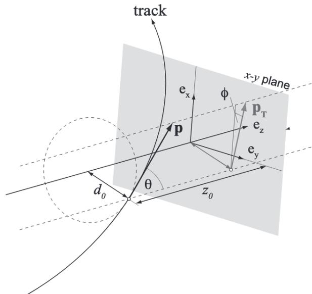
Figure 5.1.2.: Track parameterisation: A trajectory of a charged particle in a magnetic field requires five track parameters. Image from Ref. [70].
