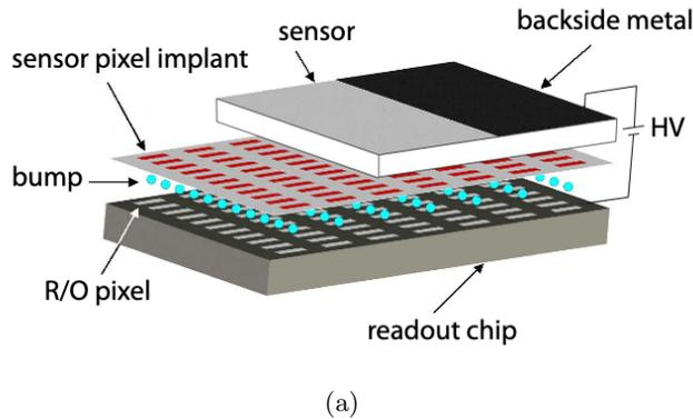
Figure 3.3.4.: The sensor and electronics chip (readout chip) have pixels of the same size, bonded to each other by means of bump contacts. Each read-out pixel corresponds to a front-end channel. Image from Ref. [34].
