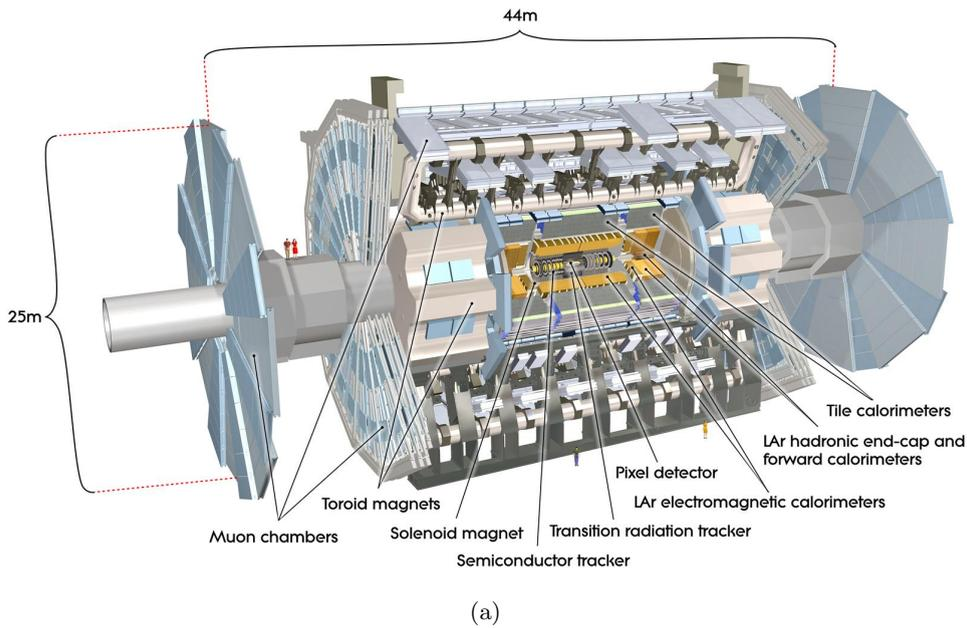
Figure 3.3.1.: ATLAS detector. Image from Ref. [28].
