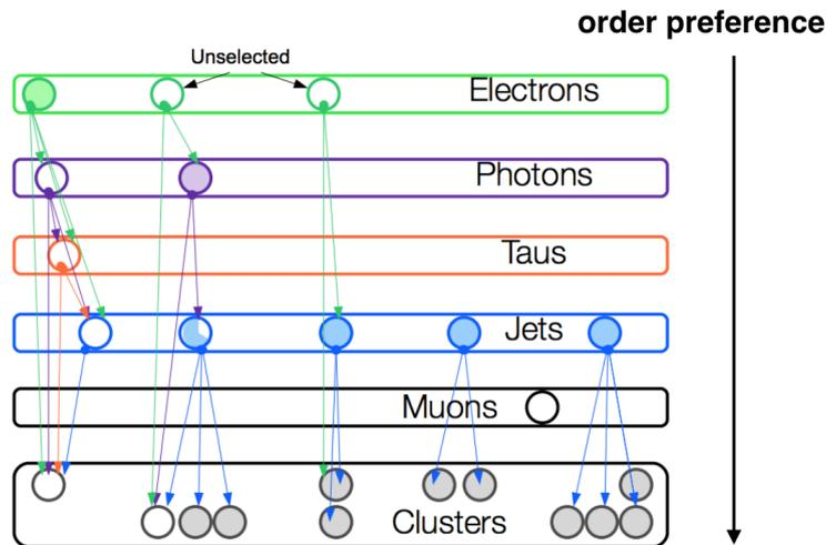
Figure 5.6.1.: Matching procedures used in the  $E_T^{\text{miss}}$  map to avoid double counting. Each circle stands for a cluster. The solid circle in green, purple, and red means the cluster is matched with the object. The cluster is then removed if it is associated with an object, otherwise the cluster is recognized as a jet in blue. The lines link between clusters and objects through a  $\Delta R$  matching [99].
