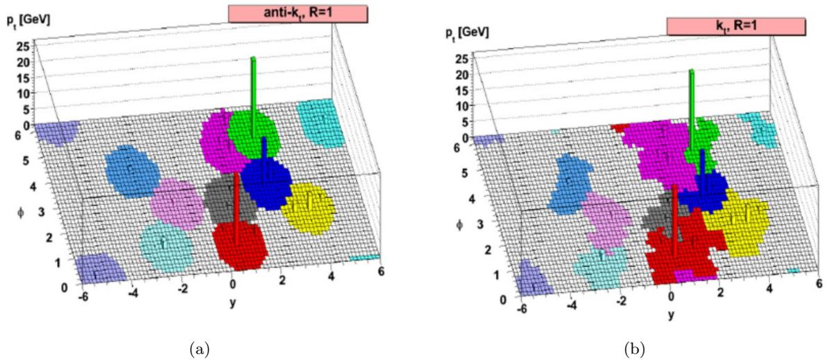
Figure 5.4.1.: Coloured areas represent clustered jets. An illustration of the  $anti-k_t$  jet reconstruction is shown on the left and  $k_t$  algorithm is shown on the right. The preference for hard radiation can be seen in the features of  $anti-k_t$  jets [78].
