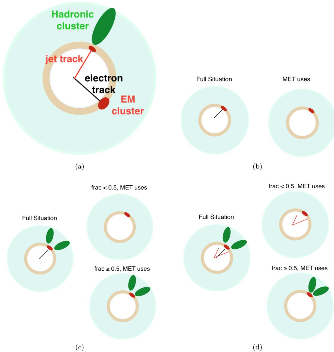
Figure 5.6.3.: Illustration of the old treatments used for the overlap removal in the  $E_T^{\text{miss}}$  calculation. (a) Legend. (b) Only one electron and no jet. (c) Only one electron and one jet without jet tracks. (d) Only one electron and one jet with jet tracks.
