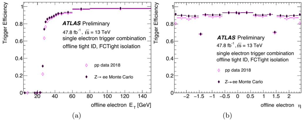
Figure 6.1.1.: Efficiency of the lowest un-prescaled single electron trigger combination (logical OR of HLT\_e26\_lhtight\_nod0\_ivarloose, HLT\_e60\_lhmedium\_nod0 and HLT\_e140\_lhloose\_nod0) in 2018 data, compared to  $Z \rightarrow ee$  POWHEG +PYTHIA Monte Carlo (a) as a function of the offline electron transverse energy, (b) as a function of the offline electron pseudorapidity. The offline electron fulfills a tight offline identification requirement. Image from Ref. [107].
