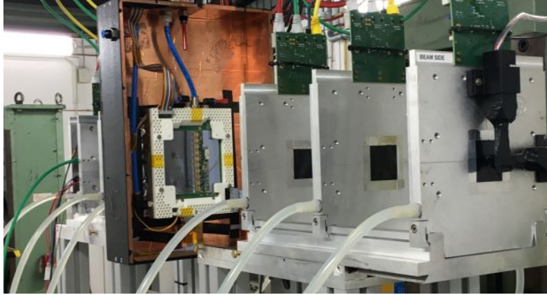
Figure 4.2: Test beam set-up in June 2018. The cooling box is open to show the ITk Strip module under test.
