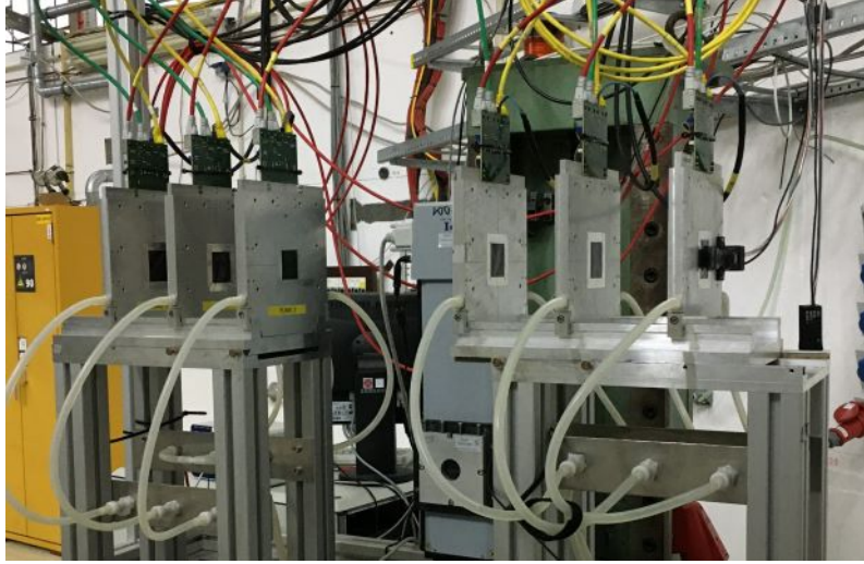
Figure 3.4: The DURANTA EUDET-type telescope installed at the test beam area T22 of the DESY II test beam facility. The six telescope planes are visible, with the active Mimosa26 sensors being located at the center of the planes behind a black kapton tape. The pipes on the side transport water to cool the Mimosa sensors. The Mimosa sensors are read out by the boards on top of the telescope planes, which also provide the trigger interface. The black scintillator in front of the first plane provides the triggers for the whole set-up.
