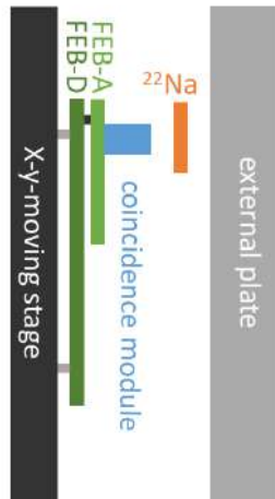
Figure 6.13: A sketch of the optimization setup.
