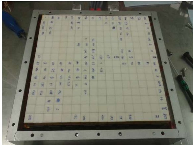
Figure 3.5: View into the open external plate. The individual modules are visible, each under a teflon cap.
