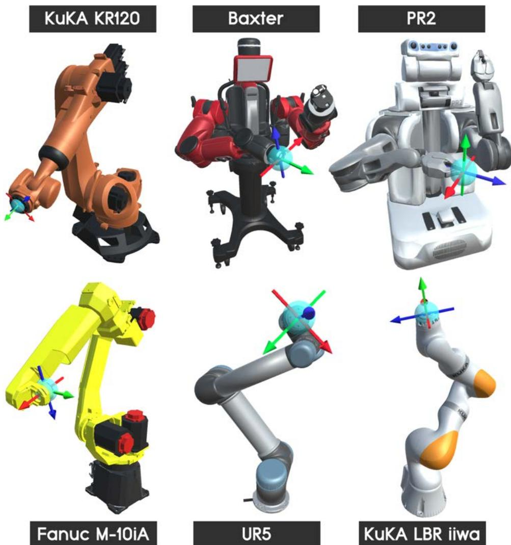
Figure 5.5: Robot models for the experimental results listed in Tbl. 5.2. The teal spheres visualise the Cartesian pose targets for solving inverse kinematics.
