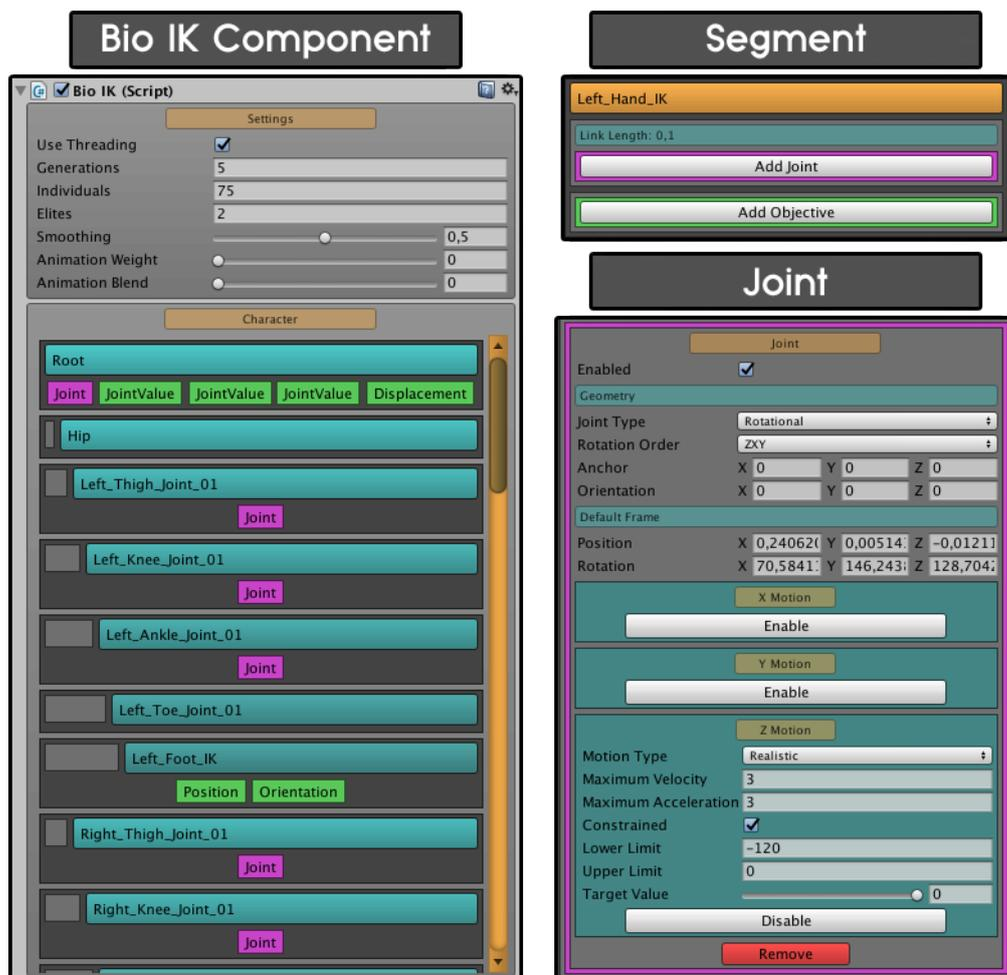
Figure 4.15: Main component and inspectors for the Bio IK asset in Unity3D.
