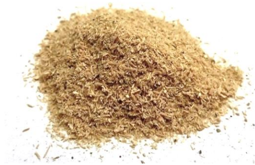
Figure 12: Hammer mill produced particles from Ethiopian highland bamboo (Stute 2018)
