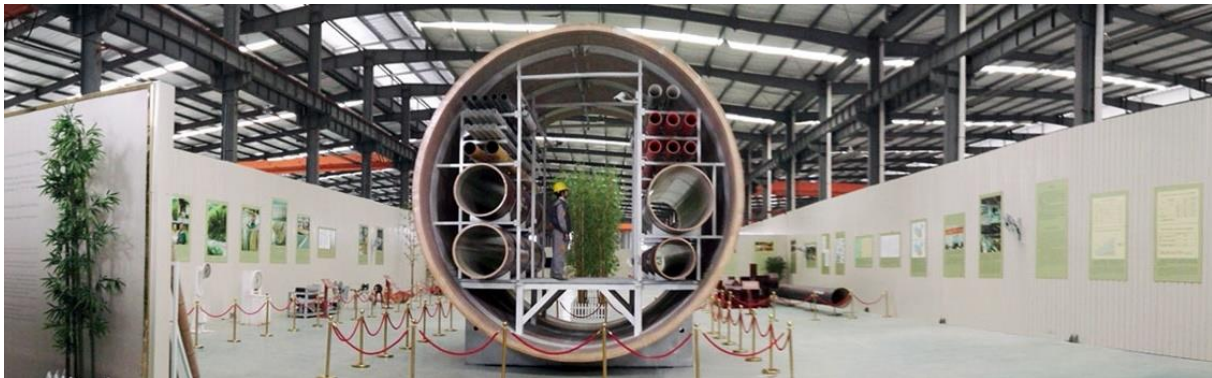
Figure 9: View on infrastructure utility tunnel made from a bamboo-based winding composite (XZBBC 2016)
