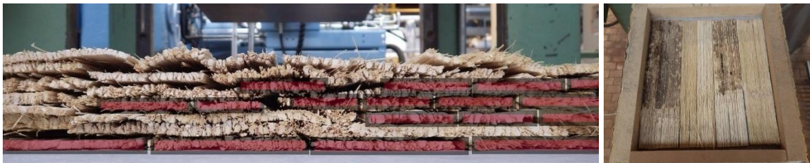
Figure 58: Mat formation with narrow scrim in the core, medium strands in the center and broad strands in the face layer (left) using a softboard template (right)
