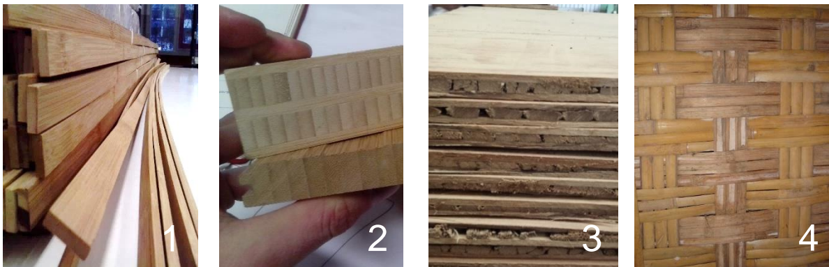
Figure 21: Planed moso slats (1) for Chinese glue laminated bamboo lumber (2) and Colombian ply boards made from raw guadua strips (3) and a hand woven highland bamboo mat produced for Ethiopian vernacular construction (4)
