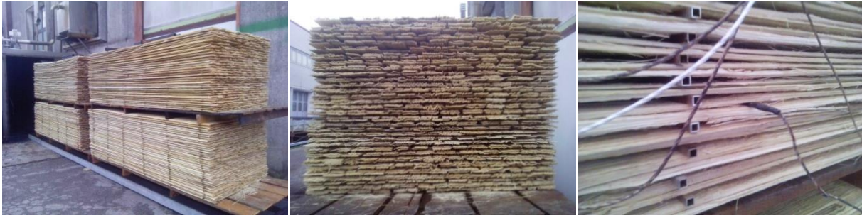
Figure 74: A chamber-ready batch of manually stacked scrim strands with 20 mm spacing and 20 mm layer thickness separated by aluminum spacers
