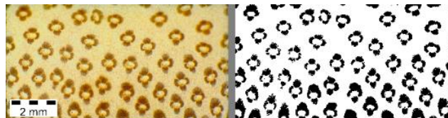
Figure 36: Microscopic image and processed binary image of a compression sample cross section
