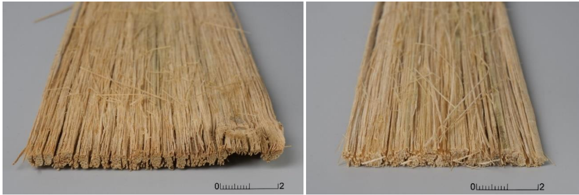
Figure 68: Scrim strands from the top portion (left) and fine crushed scrim from the same top portion (right)
