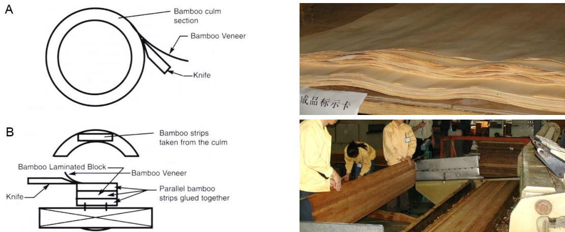
Figure 20: The two most common bamboo veneer production methods (left): Rotary slicing of a culm (A) and fineline block-slicing (B), adopted from Hidalgo López (2003) and a Fineline veneer industrial plant in Hangzhou, Zhejiang (right), adopted from Fu (2008)
