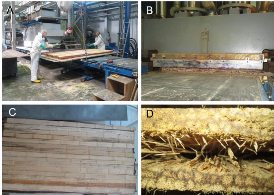
Figure 72: Manual fiber bundle layup (A), hot press compression (B), finished bamboo scrimber panel (C) and blow-out in the cross section from the industrial scale pilot production
