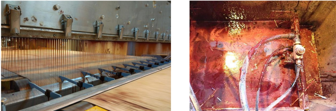
Figure 60: Resin application by liquid extrusion gluing pushing the glue paste through several fine nozzles composing a pseudo-curtain (left) and the bottom side of the circular jet gun station atomizing the resin solution with pressurized air (right)
