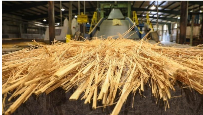
Figure 14: The scrim after being released from the crusher line (Hemmings 2019)
