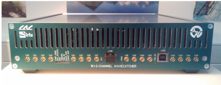
Figure B.12: The photo of the 16 channel WaveCatcher digitizer used for the tests of the straw tubes. The figure is adapted from [96].
