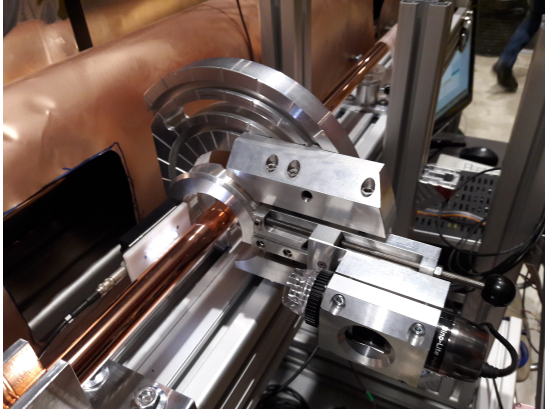
(a) Optical setup installed around the short straw tube. The digital microscope is visible on the right, the LEDs on the left (opposite side of the straw).
