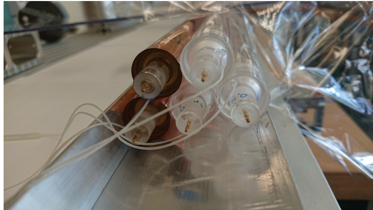
Figure 2.1: The image of 5 straw tubes glued together à la PANDA STT design [50].
