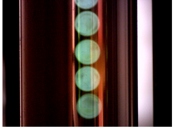
(b) Sample image obtained from the digital microscope. The shadow of the wire can be observed in the middle of the tube and is highlighted by the LED spots.
