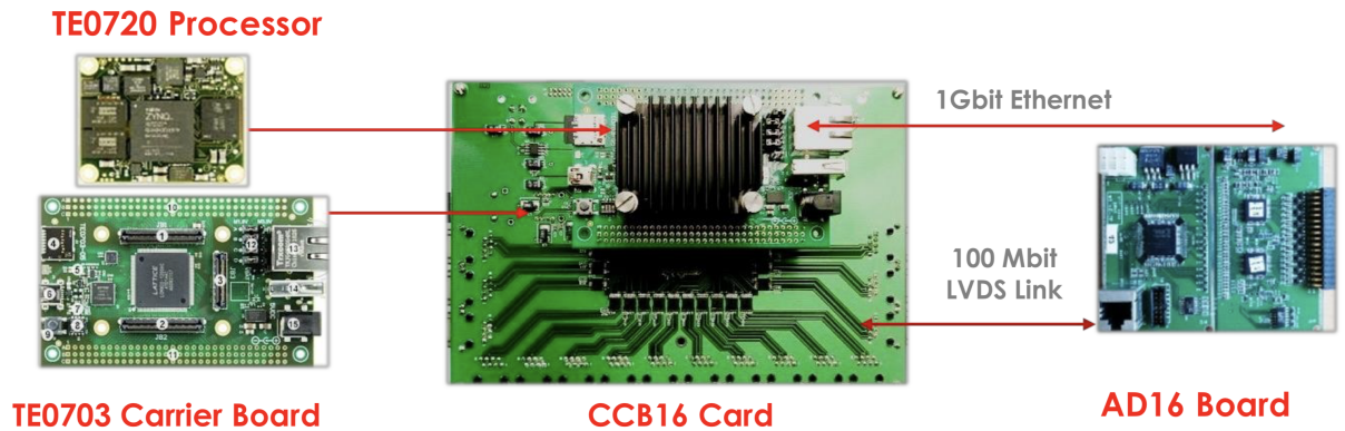
Figure B.1: The images of the AD16 front-end card and the CCB16 concentrator board. The interface connections between the boards are shown schematically too 1 .
