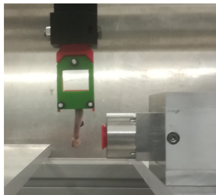
Figure 8.1 – Experimental setup with rat thigh bone in 3D printed mount and detector at the right.
