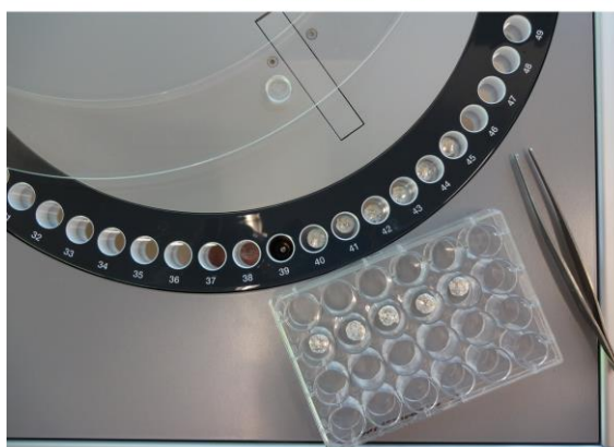
Figure VII-22: Photographic documentation of specimen preparation for elemental analysis by means of the Figure VII-21 device as described in Chapter IV–2.4.1, with milled particles (top), labMDF shavings made by fine-toothed saw, weighing and packing in thin tin foil, and sample feeder loading.
