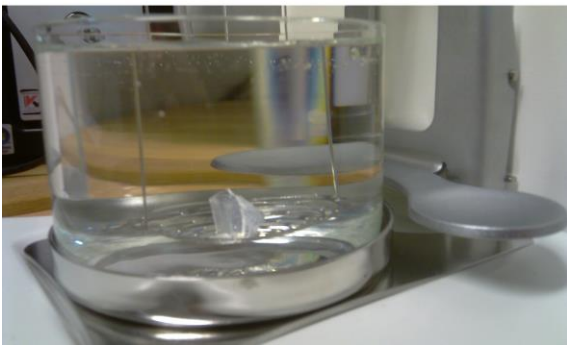
Figure VII-12: Analysis equipment for additional density determination on dry adhesive resin by means of immersion method following DIN EN ISO 1183-1 (2013) via Archimedes' principle (i.e. buoyancy method) with purified water (without wetting agent) as immersion liquid (IL), with analytical balance XS205DU, Mettler-Toledo GmbH, Giessen, Germany, equipped with the corresponding density kit.
