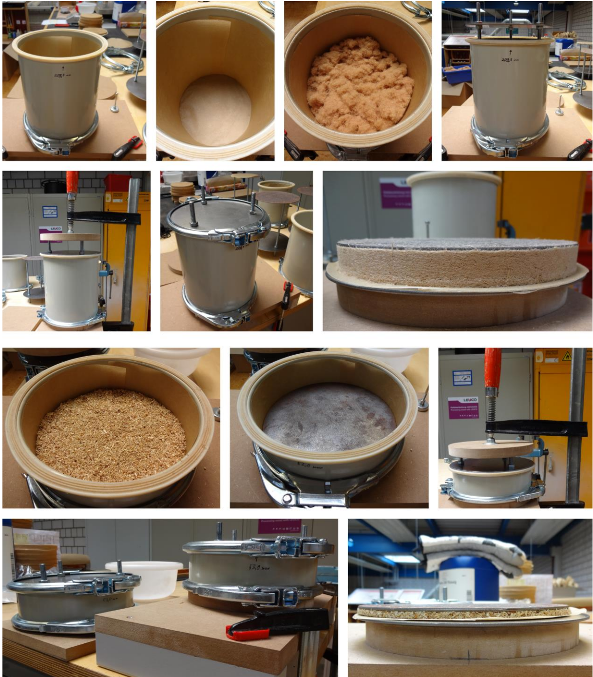
Figure VII-1: Photographic documentation of the densification setup for manufacturing of lab-made furnish mats (Chapter IV–1.1) with exemplary photographs for Fmat2 (top) and SLmat (bottom).
