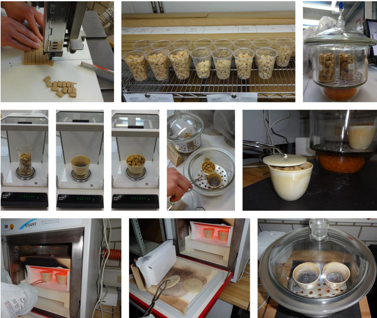
Figure VII-19: Photographic documentation of the ash content determination procedure via complete combustion according to Table IV-10.
