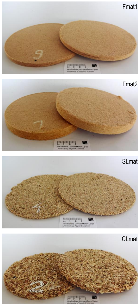
Figure IV-2: Final lab-made furnish mats as cured disk-shaped bodies made of resin-blended TMP fibres (top and middle, henceforth labelled Fmat), SL (middle, SLmat), and CL (bottom, CLmat) particles.
