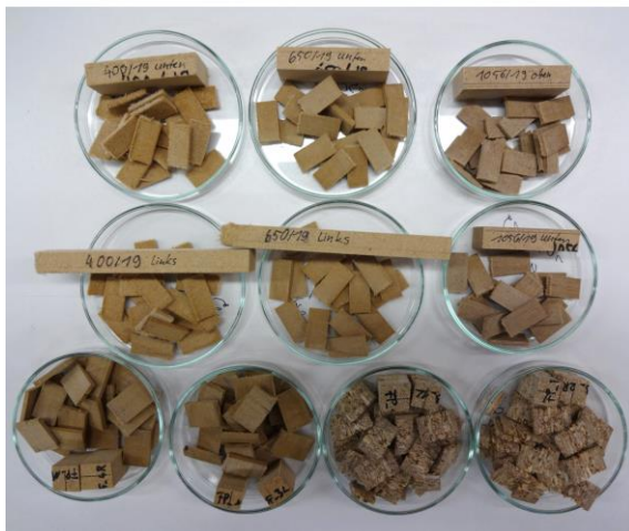
Figure VII-10: Sample preparation for true density determination via gas pycnometry on panel material with 10 mm wide parallel offcuts (top), cutting of single specimens by band-saw with nominal dimensions of 2 \dots 3 \times 10 \times 19 \text{ mm}^3 ( l \times w \times t_{\text{panel}} ) (middle), and randomly mixed material (bottom); for fibrous material see Appendix VII-2.2.
