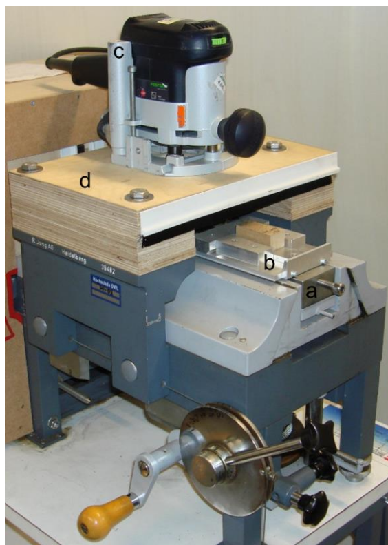
Figure IV-15: Setup of the gravimetric reference method with slide of the modified microtome (a), sample holder with specimen (b), hand router Festool OF 1000 (c) incl. face milling cutter ( \varnothing 30 mm), and baseplate (d) to fasten router instead of knife block.
