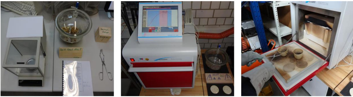
Figure VII-18: Analysis equipment for ash content determination via complete combustion according to the procedure in Table IV-10, with analytical balance AE240, Mettler-Toledo (left), desiccator, microwave laboratory system StarT Pyro T-1640, MLS GmbH, Leutkirch, Germany as exhaust air high-temperature furnace (middle and right) complete with porcelain combustion crucibles with lid.
