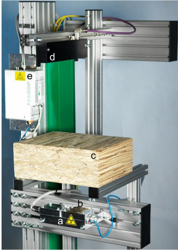
Figure IV-14: Exemplary W\text{-mat-}\rho_A setup of the W -target device with X-ray tube (a), aperture (b), any WBC specimen (c), and detector (d) as well as high-voltage generator (e), without installed pre-filters.
