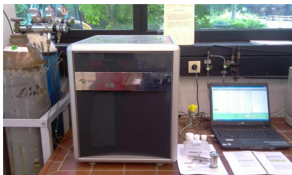
Figure VII-21: Analysis equipment for determination of mass fractions of the non-metallic chemical elements C, H, N, and S (elemental analysis) by means of the vario MACRO cube CHNS, Elementar Analysensysteme GmbH, Hanau, Germany.
