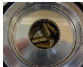
Figure VII-11: Analysis equipment for true density determination via gas pycnometry at the Institute of Wood and Paper Technology, Technische Universität Dresden, Germany with the gas pycnometer ULTRAPYCNOMETER 1000, QUANTACHROME GmbH & Co. KG, Odelzhausen, Germany complete with peripheral equipment for supply and conditioning of Helium (He) as displacement gas at 1.31 bar pressure and \vartheta_{\text{set}} = 20 \text{ }^\circ\text{C} ; exemplary specimens of lab-MDF (middle), PB-19 (bottom left), and raw TMP fibres (resin-unblended) of labMDF (bottom right) within the measuring cell.
