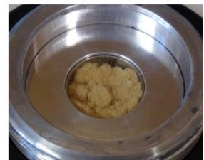
Figure VII-11: Analysis equipment for true density determination via gas pycnometry at the Institute of Wood and Paper Technology, Technische Universität Dresden, Germany with the gas pycnometer ULTRAPYCNOMETER 1000, QUANTACHROME GmbH & Co. KG, Odelzhausen, Germany complete with peripheral equipment for supply and conditioning of Helium (He) as displacement gas at 1.31 bar pressure and \vartheta_{\text{set}} = 20 \text{ }^\circ\text{C} ; exemplary specimens of lab-MDF (middle), PB-19 (bottom left), and raw TMP fibres (resin-unblended) of labMDF (bottom right) within the measuring cell.
