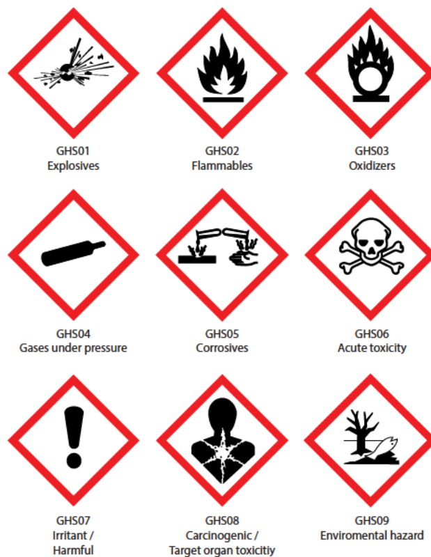
Figure B.1: Globally harmonized system of classification and labelling of chemicals. Their symbols, numbers and summarized meaning.
