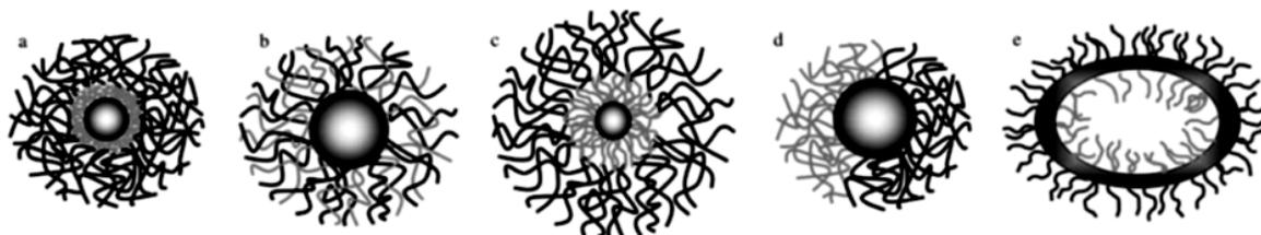
**Figure 2. 6.** Schematic representation of different types of micelles formed by ABC triblock terpolymers. Core-shell-corona micelles with a compartmentalized core (a), micelles with a mixed corona (no chain segregation) (b), core-shell-corona micelles with a compartmentalized corona (radial chain segregation) (c), Janus micelles with an asymmetric corona (lateral chain segregation) (d), and vesicles (e). Reprinted with permission from ref [99].
