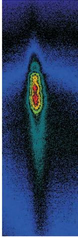
**Figure 6.6:** Fluorescence of the atoms trapped in the FORL.
