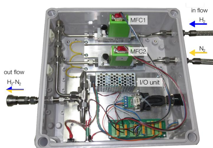
**Figure 4.9** – Two channel gas mixing device `GMS_2CH` with two Sensirion SFC5400 mass flow controllers (MFC1, MFC2) to adjust the gas flow and the mixing ratio of two gas species. MFC1 has a full scale of  $1\text{ l}_n/\text{min}$  and is used for hydrogen (blue), whereas MFC2 has a full scale of  $0.05\text{ l}_n/\text{min}$  and is used for nitrogen (yellow).
