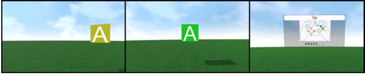
Figure 8.1.: 3DUI for the gaze-guidance experiment: (left) Unselected target. center) Selected target turned into green color after the participants kept the line-of-sight on the cube for 2 seconds. (right) Message panel with instructions for letter sequence input.
