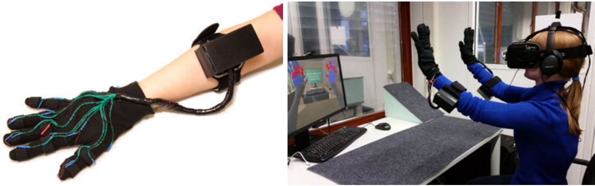
Figure 6.1.: (left) Images of the glove with the electronic case attached to the forearm, and (right) participant interacting with the VR application, wearing the pair of gloves and the Oculus Rift DK2 with the Leap Motion attached in front to facilitate the hand tracking.
