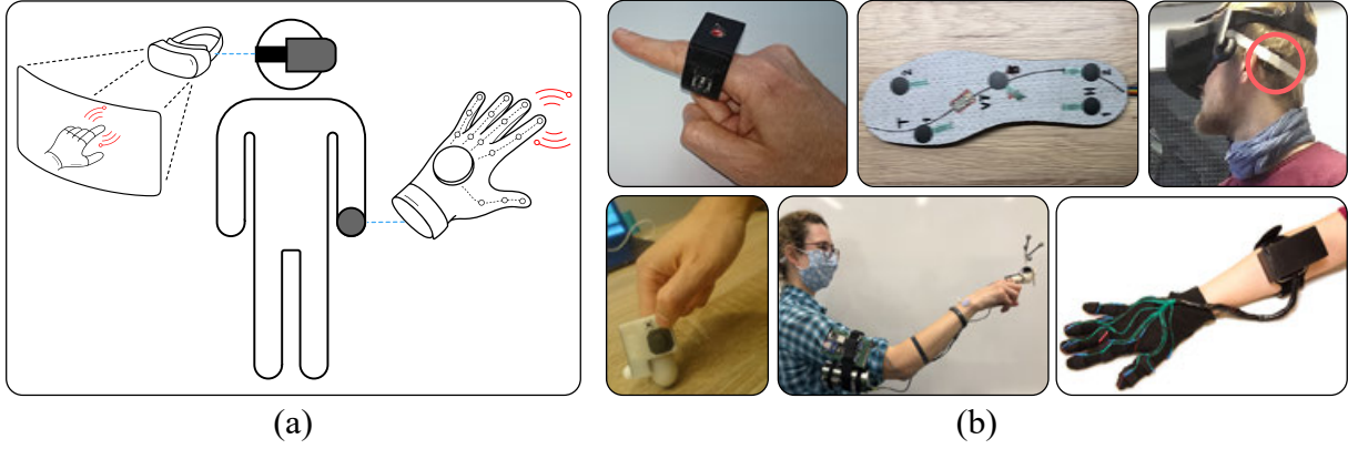
Figure 1.2.: Use of haptic wearables in VEs: (a) A user with an HMD for VR/AR applications, hand tracking is supported so the user can see a virtual representation of the real hands. The user also has a hand-worn haptic device to feel vibrations every time the virtual hand collides with a virtual object. (b) Pictures of the haptic technology that was developed in this thesis. From top-left, a trackable ring with vibrotactile feedback and digital input, a sole supporting pressure sensing and audio-based tactile feedback, a haptic module integrated into an HMD to provide gaze guidance, a wireless fingertip with analog input, gesture detection and vibrotactile feedback, a wireless device incorporating tapping sensations, piezo vibrations, and tendon/muscle electrical stimulation, and wireless haptic gloves providing tactile feedback for the palm and the fingers.
