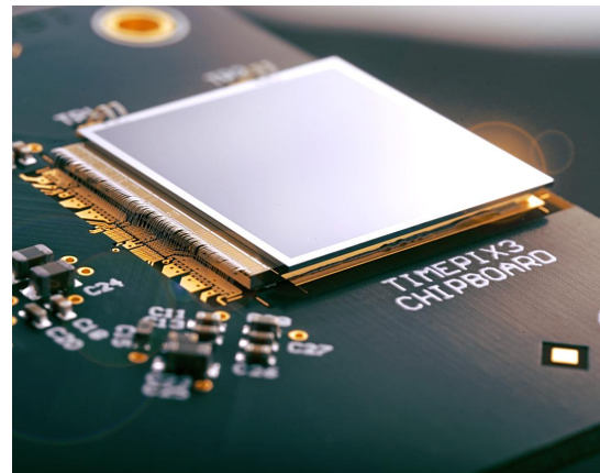
(b) Picture of the Timepix3 readout chip [27].
