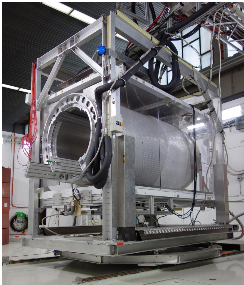
Figure 5.11 – Picture of the PCMAG superconducting solenoid located in Area T24/1 without the four additional rails used for the Lycoris telescope.
