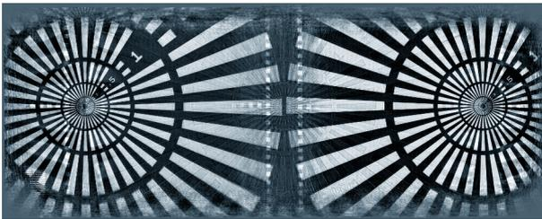
**Figure 6.9 Wrong beam distance.** Reconstructed object after 50 iterations with an assumed beam separation of  $47\ \mu\text{m}$ . Each probe faithfully reconstructs one part of the object. However, due to the wrong order of the probes, the object is reconstructed inside out.
