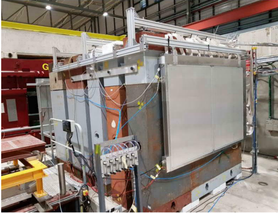
Figure 5.7: Photography of the muon tagger as seen from behind. Five planes of RPC detectors are situated between walls of iron filtering for muons [56].
