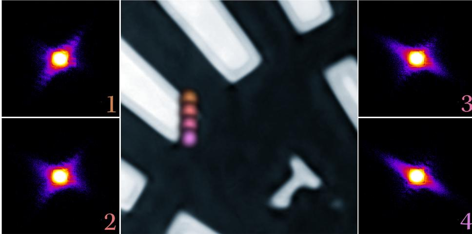
Figure 2.2: By scanning the sample with overlapping illuminations the diffraction patterns are gradually changing, thereby encoding shared information.
