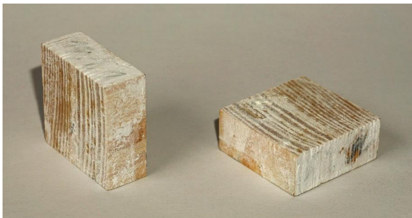
Figure 48: Solid pine sapwood samples showing thick white coating after slurry polymerization.
