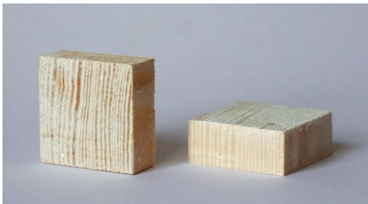
Figure 47: Solid pine sapwood samples showing white coating after the application of \text{AlMe}_3 -toluene solution.
