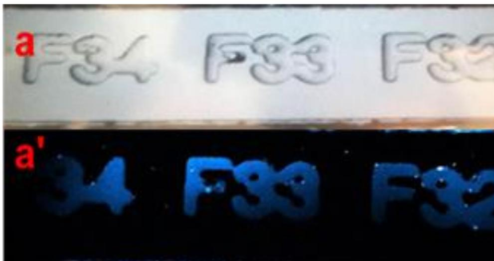
**Fig. 3-13 Bright-field and THG imaging of position labels located on a PDMS microfluidic chip.**
