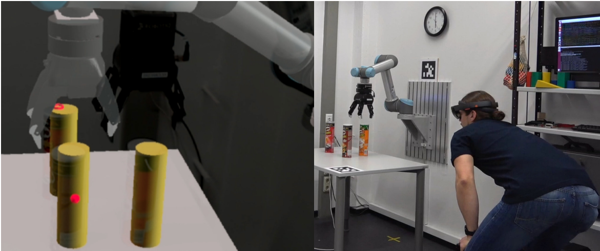
Figure 9.1: Illustration of the MR human-robot interaction: A human operator wears an optical-see through HMD for viewing the co-located robot with superimposed virtual information such as pick locations or pre-visualization of potential actions of the industrial robot arm.
