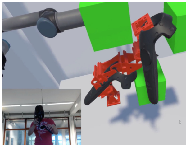
Figure 7.2: Two handed bending a modular robot into a desired posture via 6-DoF tracking of two HTC Vive controllers, which are setting a target for the BioIK instance, each.
