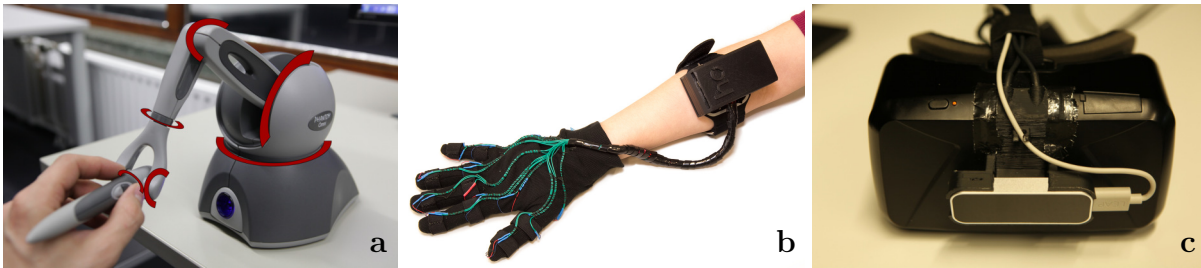
Figure B.30: Almost every input or feedback device can be integrated in own setups by writing own controller scripts based on the manufacturer’s SDK. E. g. Geomagic Touch (a), HapGlove [11] (b), HMD-mounted Leap Motion Controller (c).
