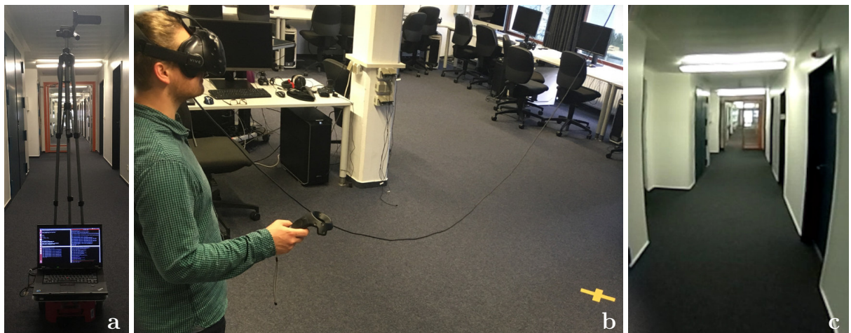
Figure 7.5: Immersive teleoperation of a mobile robot equipped with a 360° camera is based on natural walking in a VR tracking space. (a) The mobile robot (Pioneer 2-DX) is equipped with a Ricoh Theta 360° camera and operated within a building. (b) Operators see the 360° image in VR and thus, are able to decide on the viewing direction with low latency by using a dedicated shader. The robot’s motion is controlled implicitly by natural walking of the operator who is tracked within HTC Vive’s tracking space. Control commands for the robot are generated automatically and send via the ROSbridge from Unity3D to ROS running on the robot. (c) A shader implemented in Unity rectifies the image from the 360° camera in the desired viewing direction and allows additionally for small translatory movements without the need to move the camera.
