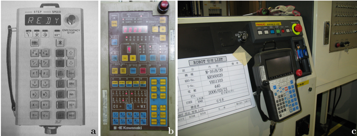
Figure 3.14: A collection of robot control hardware: (a) Robot teach box for Hobart Motoman Robot [124], (b) control panel of a Kawasaki robot from 1987 [36], (c) a recent control unit (FANUC R-J3iB Controller) of a FANUC robot [37].
