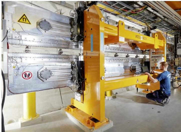
Figure (1.2) An undulator installed at EuXFEL [2].
