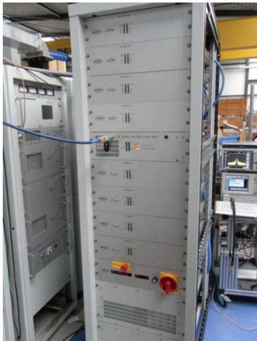
Figure (6.2) A 10 kW rack-mounted L-band SSA amplifier [101]. The rack consists of eight separate 1.25 kW modules.
