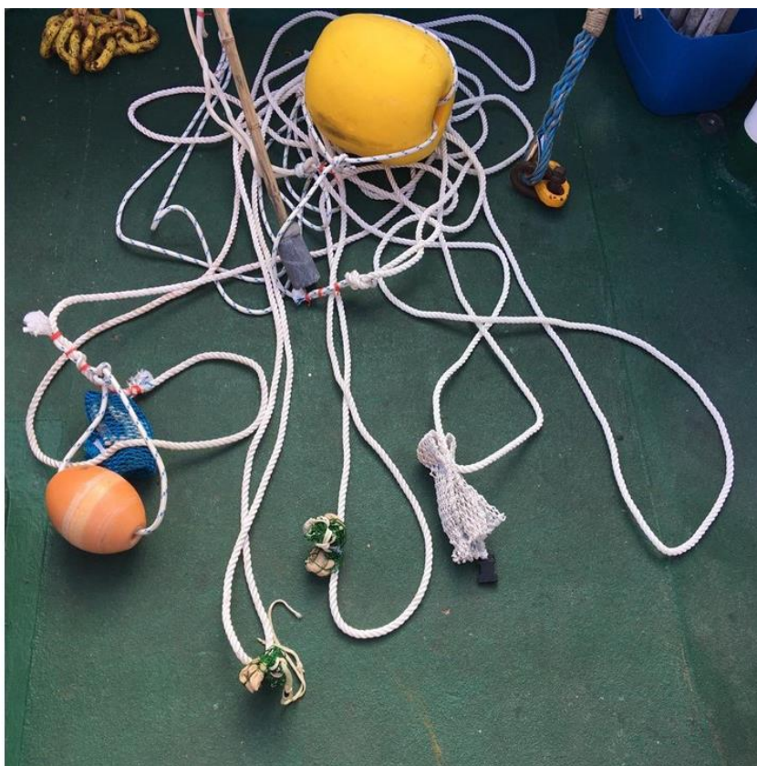
Figure S1: Photograph (left) and schematic drawing (right) of the setup of the stationary method. DSTs are mounted in small-meshed bags at around 2.5, 9 and 18 m along a rope which is marked at the surface and anchored to the bottom.
