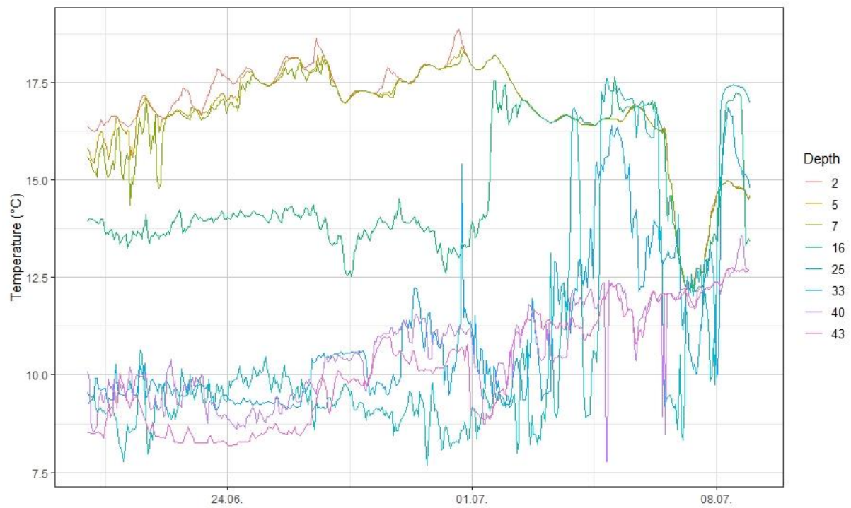
Figure S10: Temperature profiles of the automated measuring station (MARNET) in the Arkona Basin. Temperature values below 7.5 °C were deleted from the dataset since they can be accounted as measurement errors.
