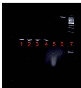
**Fig. 5** Extraction of genomic DNA from raw sample at room temperature, after rehydration of dry stored lysis buffer on microfluidic origami device. Gel lane description given in Table 2.
