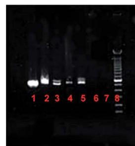
**Fig. 4** Extraction of plasmid DNA from raw sample at room temperature, after rehydration of dry stored lysis buffer on microfluidic origami device. Gel lane description given in Table 1.
