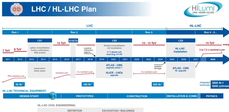
FIGURE 10.3: Schedule of the LHC and HL-LHC operations. Taken from Ref. [207].
