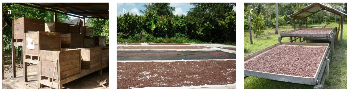
Figure 7: Fermentation and drying facilities in Peru with a box stair fermentation facility; b open solar drying on tarpaulins; c solar drying on wooden tray trolleys with rain protection.
