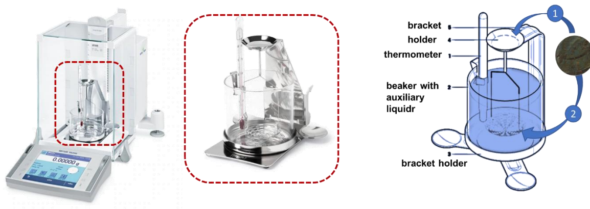
Figure 355. Balance and density kit with sketch of the density kit including description of each part. Reprint with permission from Mettler-Toledo.
