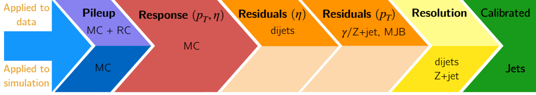
Figure 3.4.1: Simplified representation of the factorised approach used for jet calibration in CMS. More information on each step is given in the text. Adapted from [148].
