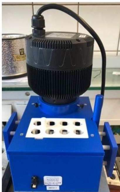
**Figure 3.** EvoluChemTMPhotoRedOx reactor fitted with a 455 nm high-power single LED.
