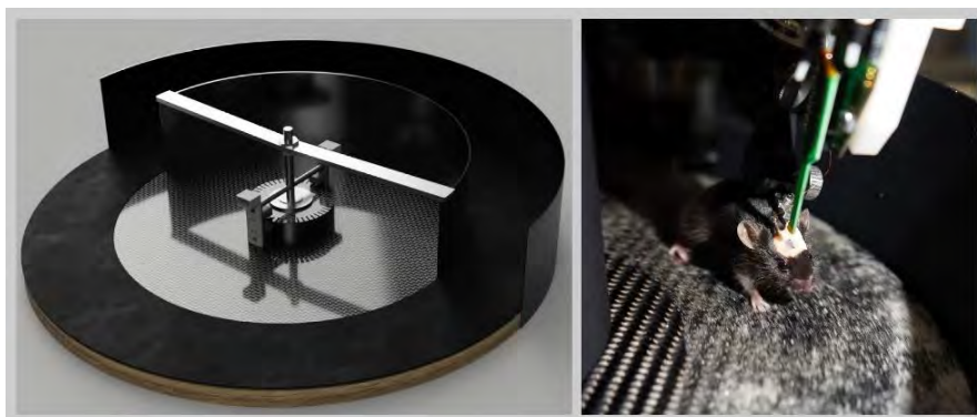
Figure 1. Establishment of chronic head-fixed recordings in developing mice using a custom-made spinning-disc setup. Left, schematic of spinning-disc setup design. Right, photograph of a P23 mouse during head-fixed recording on implemented spinning-disc setup.
