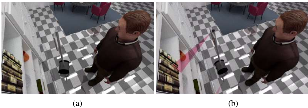
Fig. 5.1 Comparison of two telepresence systems in the perspective of bystanders: (a) Traditional telepresence robot: the host could localize a guest’s gaze directions by the rotation of platform, but the head or face of the guest is invisible in some situations. (b) 360° telepresence robot: in 360° video-based telepresence, the teleoperator (guest) has a 360° video sphere surrounding them on the HMD, so the robotic platform does not need to rotate when he or she looks around.
