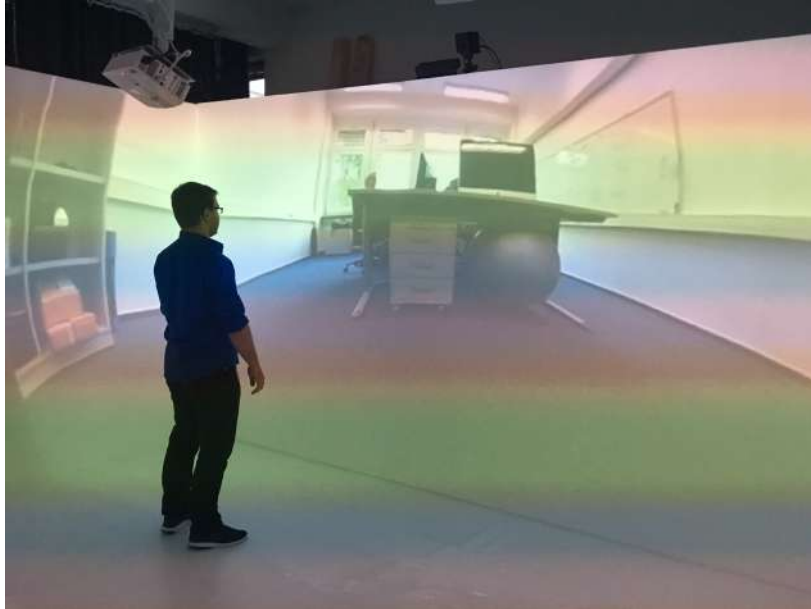
Fig. 3.8 Real-time 360° RE rendered and projected in a CAVE-like space.
