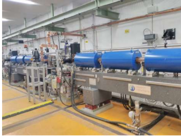
Figure 3.10.: Travelling wave structure after the gun. Solenoids around TWS are enclosed in blue casing.
