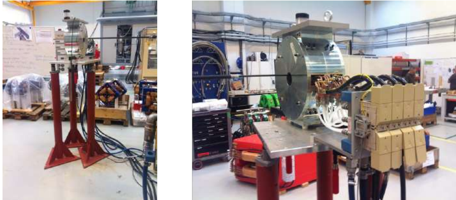
Figure 4.4.: Solenoid magnet at the manufacturing site while doing magnetic measurements. Picture courtesy Danfysik [67].
