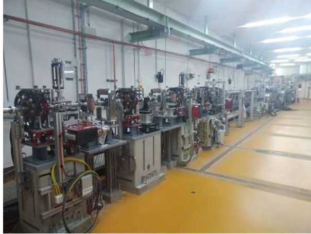
Figure 3.12.: Quadrupoles installed downstream the TWS for focusing and matching into the experimental area.
