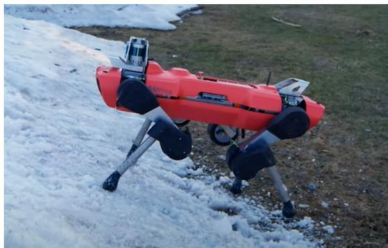
**Figure 2.7:** Using reinforcement learning to control quadrupedal over challenging terrain [71].
