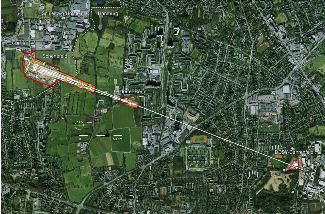
FIGURE 1.7: XFEL facility from above crossing the border of the federal county. The electron gun is located at the DESY campus in Bahrenfeld, the undulators and photon beam lines are in Schenefeld. The over all length is 3.4 km. (Source: [27])
