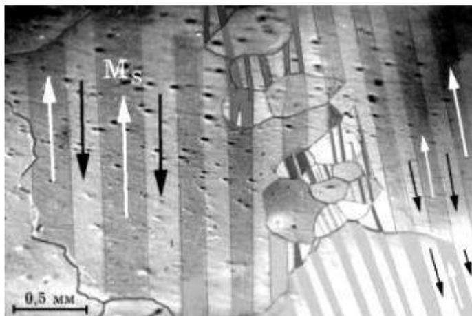
FIGURE 2.3: An interesting image shows grains and structure of magnetization (domains) of iron in the above figure, published in [59].
