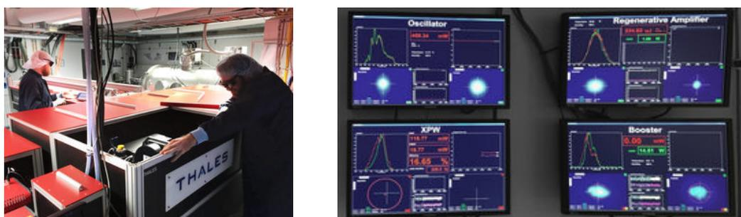
FIGURE 2.10: The laser system of the LUX group operates an 200 TW, 25 fs laser named *ANGUS*, which could run with a repetition rate of up to 5 Hz. The focus on design of laser system and beam line was on reliability and reproducibility. A high degree on automatization, such as auto-alignment procedures and continuous data acquisition including environmental conditions, enables a stable every-day operation with a high statistical determination of experiments. (Source: [90])
