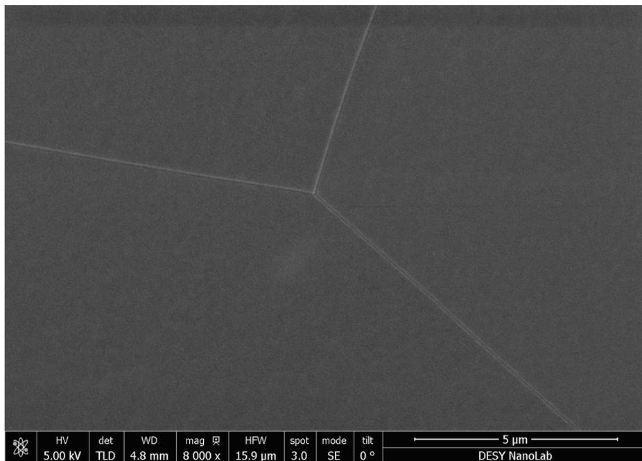
Figure 52: SEM image of EP'ed fine-grain-sample surface after 2nd 400°C nitrogen infusion.
