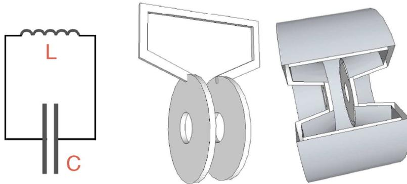
Figure 3: Cavity representation as an LC circuit [11].
