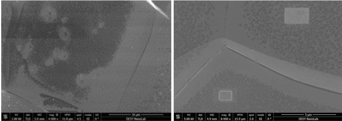
Figure 75: SEM image of sample placed without LOS protection and thus exposed to the furnace vacuum during 800°C baking.
