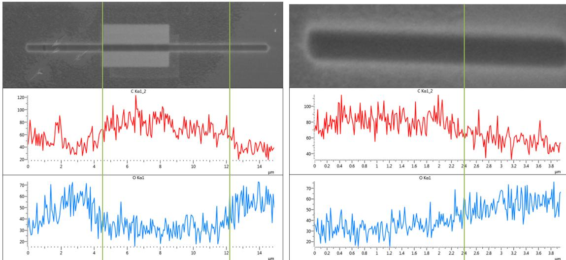
(b) EDX line scan of Spot 1 on a dark area that has been pre focused on which appears as the brighter area. (c) EDX line scan of Spot 2 at the edge of a dark window in the middle.
