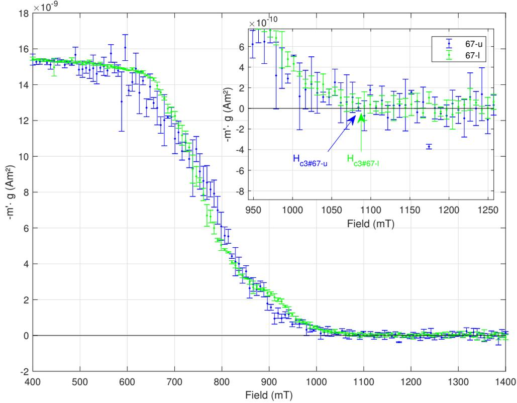
Figure 84: Negative real part of the alternating-field susceptibility measured on samples 67-u and 67-l. The surface nucleation field  $H_{c3}$  determined by the onset of excess shielding  $m' - m'_{normal}$  where  $m'_{normal}$  is the real part of  $m$  in the normal state, is indicated by the arrows. The results are re-normalized by multiplying with a weighting factor  $g = m_U / (2 \cdot m_{67-u/l})$  with the masses given in table 11.
