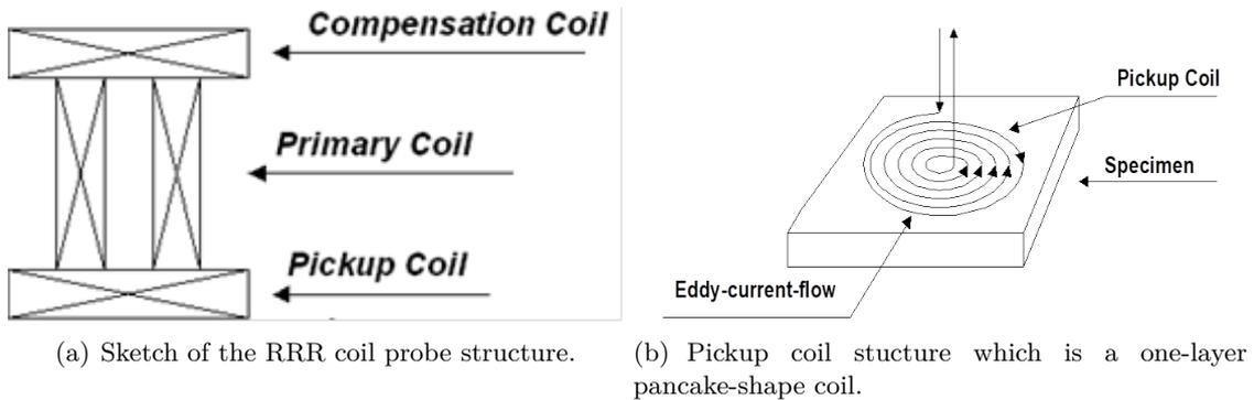
(a) Sketch of the RRR coil probe structure.
