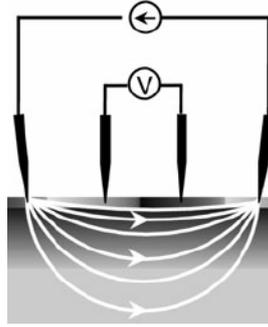
Figure 44: Illustrative principle of the 4-pt contact method [102].
