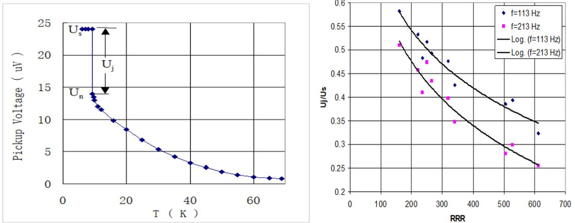
(a) Example curve of measured Pickup voltage vs temperature.
