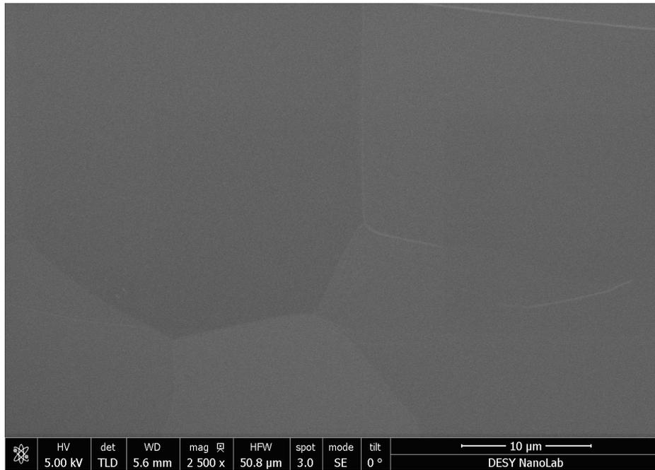
Figure 51: SEM image of EP'ed fine-grain-sample surface after 400°C nitrogen infusion.
