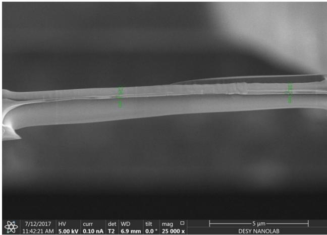
(c) SEM image with top view of the prepared lamella cut with the FIB lift-out technique from the prepared area shown in (b).
