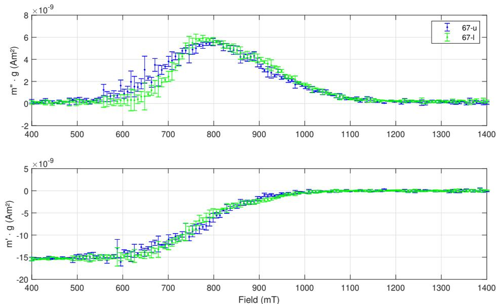
Figure 83: Real ( $m'$ ) and imaginary part ( $m''$ ) of the alternating-field susceptibility measurements of the upper half (u) and the lower half (l) of sample 67. The results are re-normalized by multiplying with a weighting factor  $g = m_U / (2 \cdot m_{67-u/l})$  with the masses given in table 11.
