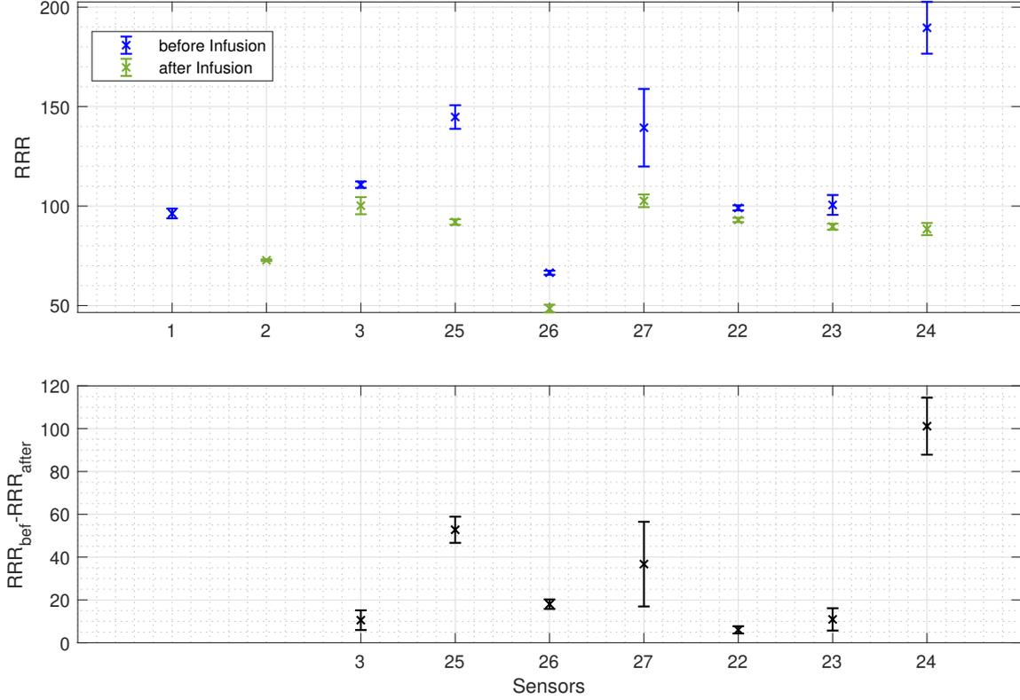
Figure 37: Measured RRR values on a single cell cavity before and after a nitrogen infusion by AC eddy current. The values are averaged over several temperature cycles. Due signal interference one of the data points for sensor 1 and 2 is missing for each measurement. The relative difference between before and fter treatment is shown in the bottom. They are in reasonable agreement except for sensors 25 and 24.
