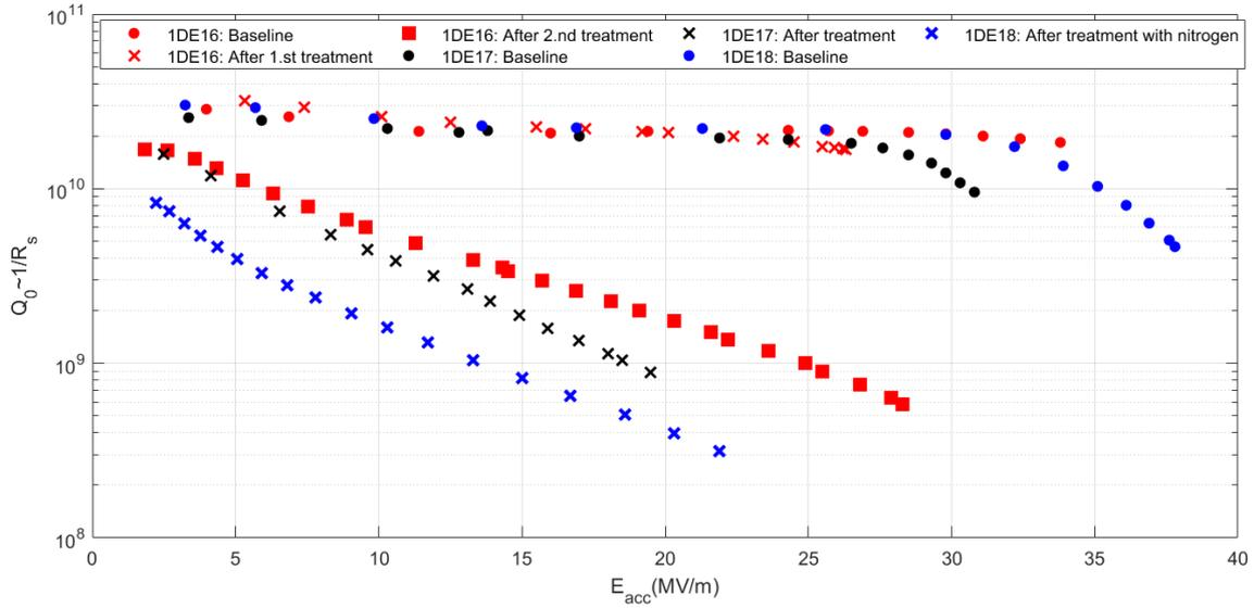
Figure 56: Cavity performance after the first attempts of heat treatment without subsequent chemical surface removal on three single-cell cavities 1DE16, 1DE17 and 1DE18 at DESY. Performance before the treatment is shown in the baseline curve for each cavity. All curves shown are taken at 2 K.
