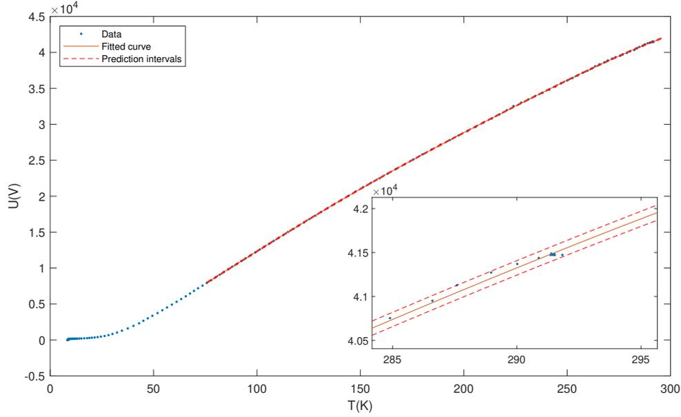
Figure 47: Data (voltage vs. temperature) from resistivity measurement of one sample from room temperature to below  $T_c$ . The error bars are smaller than the symbol size. The cubic polynomial is shown in red extrapolated to 295 K with 95% prediction intervals.
