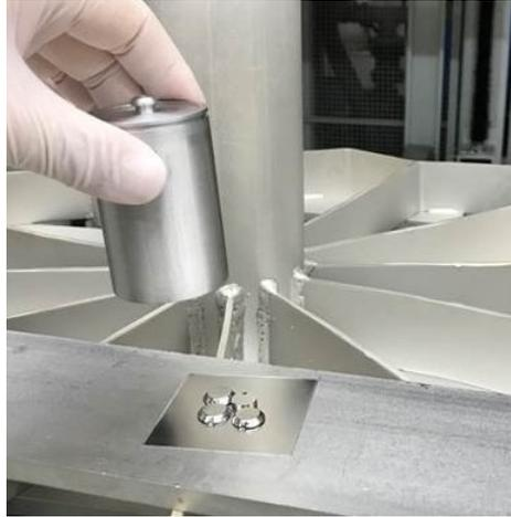
Figure 57: Coverage of cavity witness samples beneath a HOM-coupler housing as a protection against particle contamination from the oven surface in the line of sight (LOS) to the sample surface. In total, four samples are placed on a thin niobium sheet and the HOM coupler placed over them.
