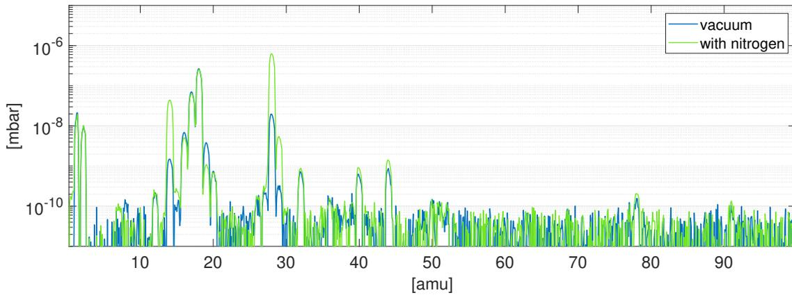
Figure 22: RGA spectrum at room temperature with and without the addition of nitrogen. In vacuum (blue) at a pressure of  $2 \cdot 10^{-7}$  mbar recorded from WRG2. With nitrogen (green) where the gas-flow controller is set via WRG2 to a nitrogen partial pressure of  $5 \cdot 10^{-7}$  mbar.
