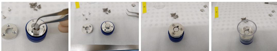
Figure 17: Mount of conical sample in aluminum pin stub holder. The aluminum pin stub is placed in a transport tube for storage, shipping and transport. It protects the samples from contamination.
