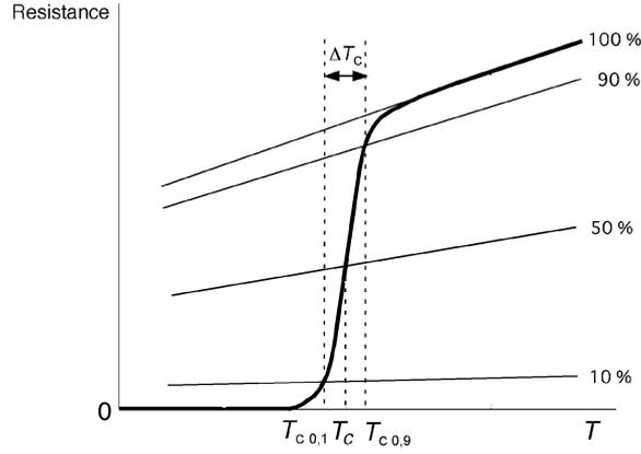
Figure 78: Determination of  $T_c$  [118].
