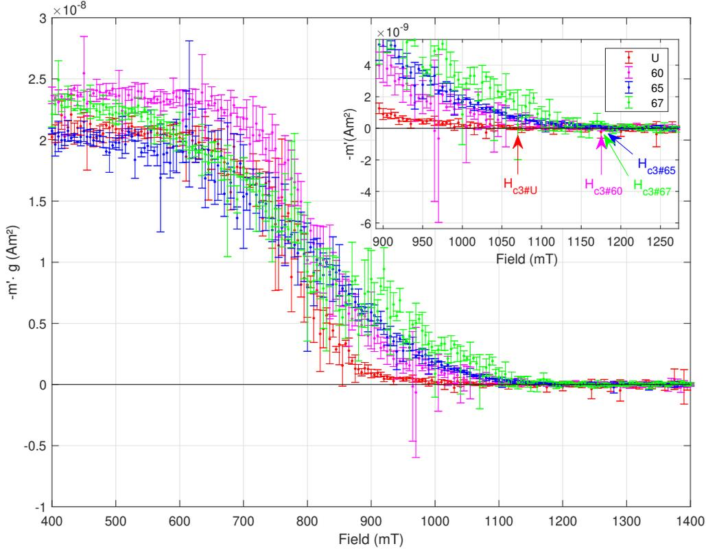
Figure 82: Negative real part of the alternating-field susceptibility measured on samples U, 60, 65 and 67. The surface nucleation field  $H_{c3}$  determined by the onset of excess shielding  $m' - m'_{normal}$  where  $m'_{normal}$  is the real part of  $m$  in the normal state, is indicated by the arrows. The results are re-normalized by multiplying with a weighting factor  $g = m_U/m_x$  with the masses given in table 11.
