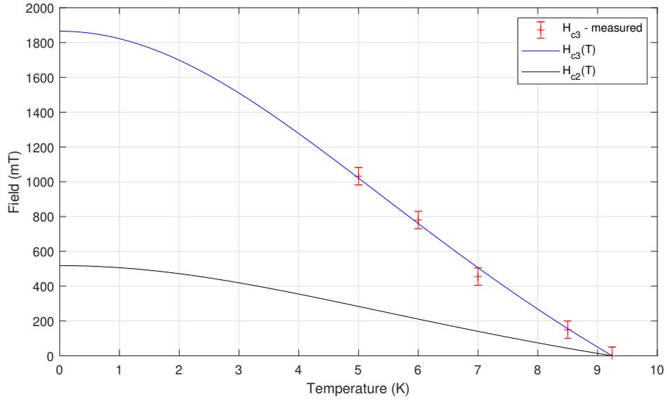
Figure 86: Measured  $H_{c3}$  of sample 67-u as a function of the temperature. Also shown is equation 16 (blue and black line) following  $H_{c2}(T)$  with  $H_{c2}(0 \text{ K}) = (518 \pm 16)$  mT from the resistivity measurement and  $H_{c3}(T)$  with  $H_{c3}(0 \text{ K}) = (1870 \pm 70)$  mT from the values obtained by the susceptibility measurement;  $H_{c3} = r \cdot H_{c2}$  gives  $r = 3.6 \pm 0.18$ .
