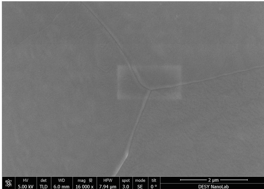
Figure 49: SEM image of EP'ed fine grain sample surface after 180°C nitrogen infusion. The grain boundaries are clearly visible while the surface has a clean smooth appearance. The rectangle comes by the charging effect from the scanning electron microscopy which is known to cause change in image contrasts [108].
