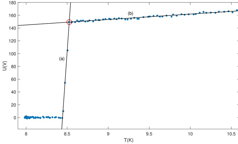
Figure 46: Data (voltage vs. temperature) from resistivity measurement of one sample and the two fitted lines (a) and (b) to determine the intersection marked by the red circle giving  $U(T_c)$ . The error bars are smaller than the symbol size.
