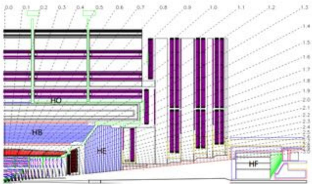
**Figure 3.6** – The layout of one quarter of the CMS HCAL. It consists of a hadron barrel part (HB) and endcap system (HE), outer (HO) and forward calorimeters (HF), covering a pseudorapidity region of  $|\eta| = 5.2$ , from [39].
