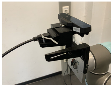
Figure 7.8 – Camera holder in active vision system.
