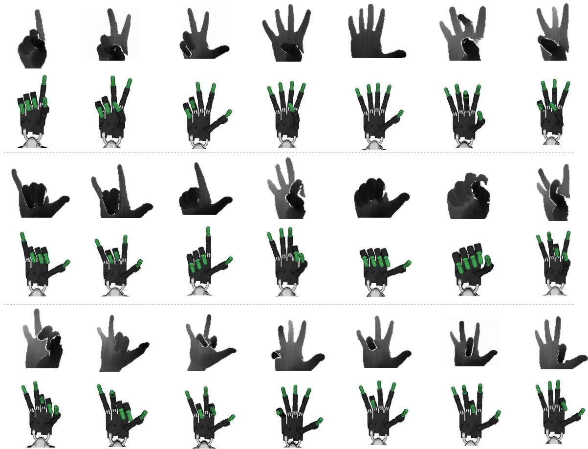
Figure 4.9 – Teleoperation results using the virtual Shadow hand with position control. The first, third, and fifth rows are depth images of the human hand captured by the Intel RealSense F200 depth sensor. The second, fourth, and sixth rows are the screenshots of the teleoperated Shadow hand in RViz.
