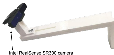
Figure 6.6 – The camera holder is used to mount the camera on the human arm.
