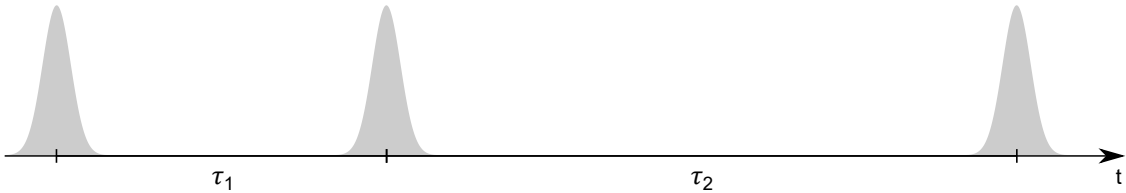
Figure 2.2: Pulse sequence used for the discussion of the third order non-linear response function. \tau_1 ( \tau_2 ) is the time interval between pulse 1 and 2 (2 and 3).
