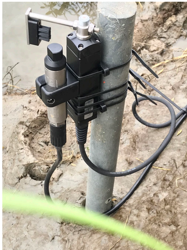
Figure 5.8 Optical backscatter sensors placed in a mainland salt marsh close to creek in order to obtain data on suspended sediment concentrations.
