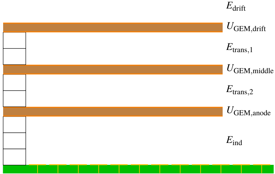
Figure 6.5.: Location of the fields and voltages in the GEM stack of the readout module defined in the text and in table 6.1. The readout pads indicated by the yellow stripes at the bottom are on ground potential.
