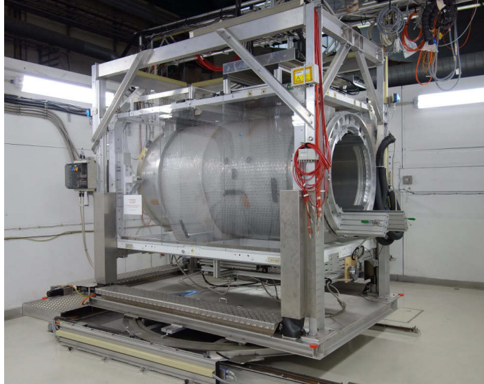
Figure 6.2.: The PCMag solenoid magnet mounted on its movable stage in the DESY test beam area T24/1. The electron beam is entering from the wall behind the magnet, perpendicular to the bore axis of the solenoid.
