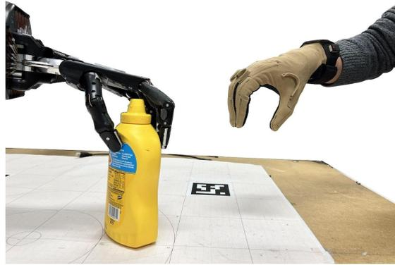
**Figure 5.3:** An illustration of human teleoperating Shadow hand using a Cyberglove for robotic grasp pose dataset collection.
