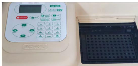
Figure 2.13: Spectrophotometer used for quantification experiments (Biorad, Model 680)
