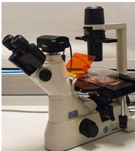
Figure 2.8: Inverted microscope used for all experiments, NIKON ECLIPSE TS100
