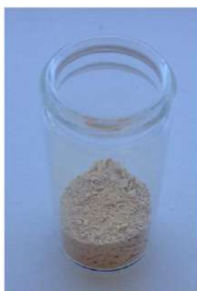
Figure S9. Poly(bisphenol A carbonate) synthesized by polymerization of bisphenol-A diacetate and diphenyl carbonate.
