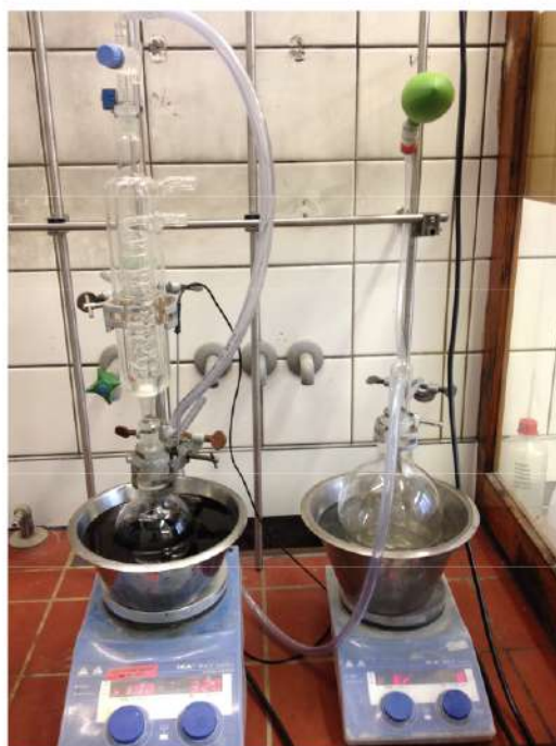
Figure S7. Reaction set up for depolymerization coupled with carbon dioxide capture.
