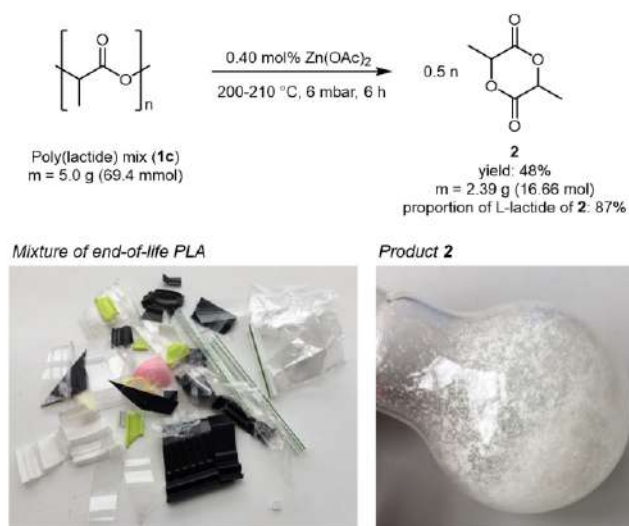
Scheme 4. Depolymerization of a mixture of end-of-life PLA (transparent cup (1 oz), transparent cup (250 mL), transparent disposable food box, transparent sushi box cover, transparent bottle, drinking straw with green strips, disposable fork with talcum powder, lid for espresso mugs (contains ~20–30% talcum powder), lid for coffee mugs, black lid for coffee mugs, sushi box (black base), ice cream spoons, foil) [Conditions: 1c : 5.0 g, 69.4 mmol with respect to the monomer unit, it is presumed that 1c is composed of 100% of PLA), Zn(OAc) 2 (0.4 mol%, 50.92 mg, 0.278 mmol with respect to the monomer unit of 1c ), 200–210 °C, 6 mbar, 360 min].
