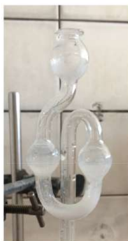
Figure S1. Detection of carbon dioxide formed during the transesterification of diphenyl carbonate with acetic acid.
