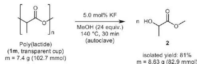
Scheme 4. Scale-up degradation of end-of-life PLA performed with conventional heating in an autoclave [Conditions: 1m (102.7 mmol), MeOH (2.47 mol; 24.0 equiv. with respect to the monomer unit of 1m ), potassium fluoride (5.13 mmol, 5.0 mol% with respect to the monomer unit of 1a ), temperature: 140 °C (conventional heating), time: 60 min].
