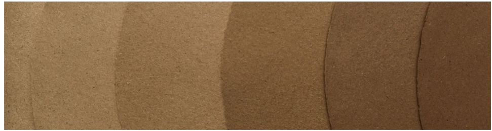
Fig. 4 Testsheets made out of SR-MDF (A) without additional beating steam treated at severities of 2.5, 2.8, 3.1, 3.4, 3.7 and 4.0 (from left to right)
