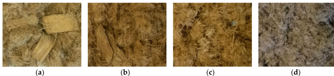
Figure 6. Morphology of poplar wood after steam refining using different treatment conditions [logR 0 ; °C; min]: (a) 2.47; 150; 10, (b) 3.06; 160; 20, (c) 3.36; 180; 10, (d) 3.95; 190; 20.
