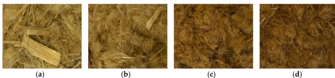
Figure 7. Morphology of spruce wood after steam refining using different treatment conditions [ \log R_0 ; ^{\circ}\text{C} ; min]: (a) 2.47; 150; 10, (b) 3.06; 160; 20, (c) 3.36; 180; 10, (d) 3.95; 190; 20.
