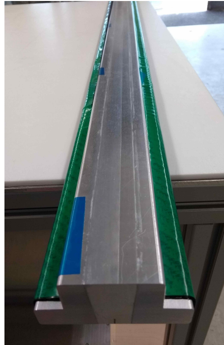
(b) Mold with one layer of prepreg around it.
