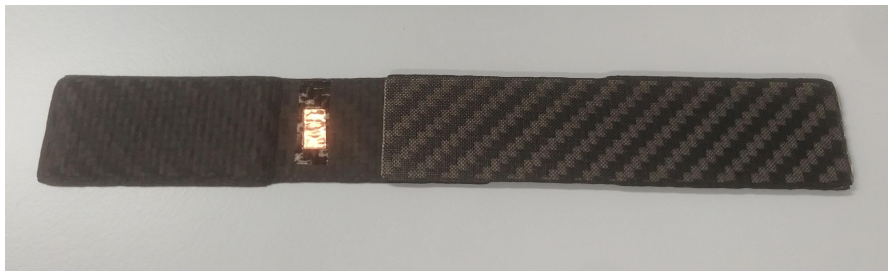
Figure 5.29: Lap joint sample after gluing.
