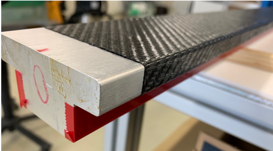
Figure 5.10: First layer of the prepreg directly placed onto the mold.
