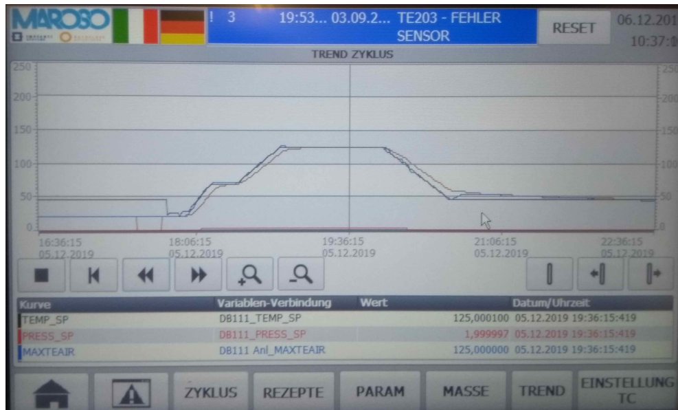
Figure 5.13: Autoclave curing cycle used for co-curing the service trays.
