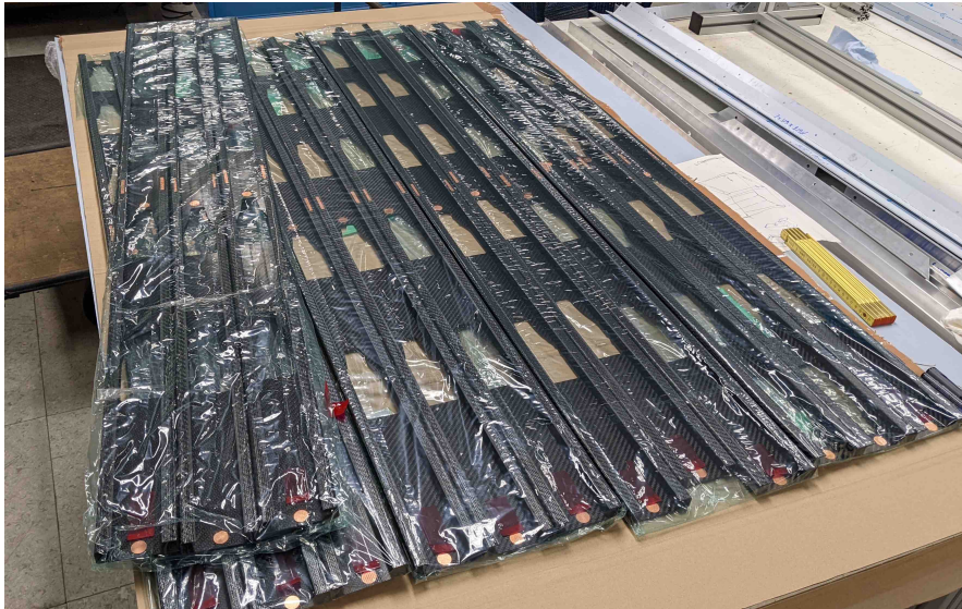
Figure 5.37: Final service trays after machining.
