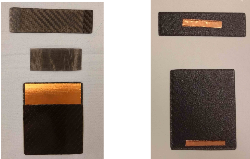
(a) Samples shown with glued surface facing upwards. The CF mat is shown in the middle. (b) Samples shown with the outside facing upwards.
