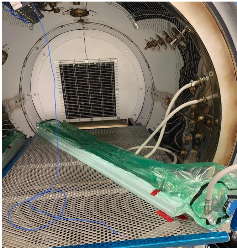
Figure 5.12: Evacuating the air out of the sealed vacuum bag.
