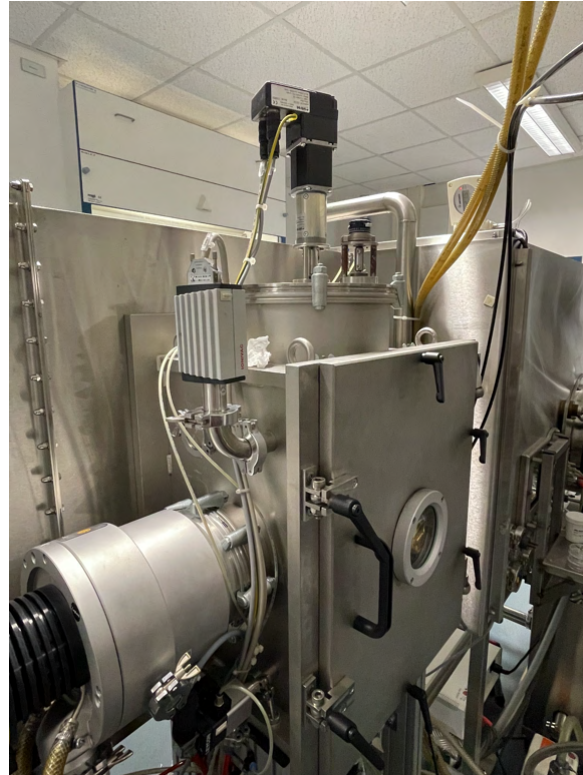
Figure 19: Equipment at Fraunhofer CAN for the PVD. The vacuum chamber is connected to a turbo pump, which allows the extraction of gas molecules in order to achieve high-vacuum. The chamber has also two inlets, allowing the insertion of materials from the outside as well from inside a glove box.
