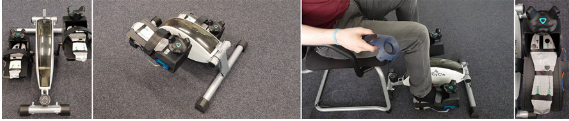
Figure 9.1: The VR Strider device including mini exercise bike and electronics for pressure tracking and vibrotactile feedback.
