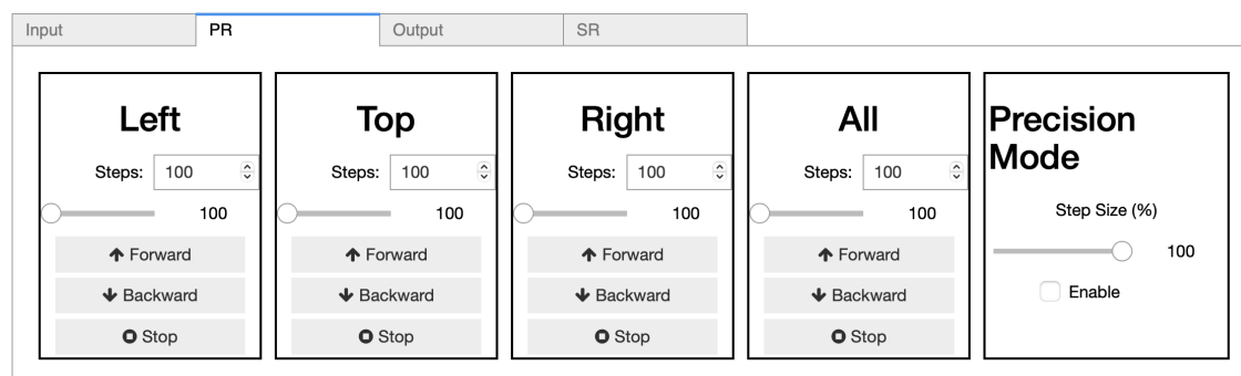
Figure D.1.: Screenshot of the GUI for the mirror positioner control software. It is build with widgets inside of an Jupyter Notebook [74] which enables cross-platform compatibility. The mirror positioners are split into multiple tabs, each displaying the piezoknobs for a single positioner. The selected tab here displays a positioner which is configured as shown in listing D.1 with an exemplary configuration. Each piezoknob is shown in its own section with a selection for the number of steps and a button for the direction. Additionally, one can move all three piezoknobs at the same time. By default, the step size is set to 100 %. By enabling the precision mode, one can tune the step size and overwrite the default value. This is useful for tuning the mirror position in a sub wavelength range.
