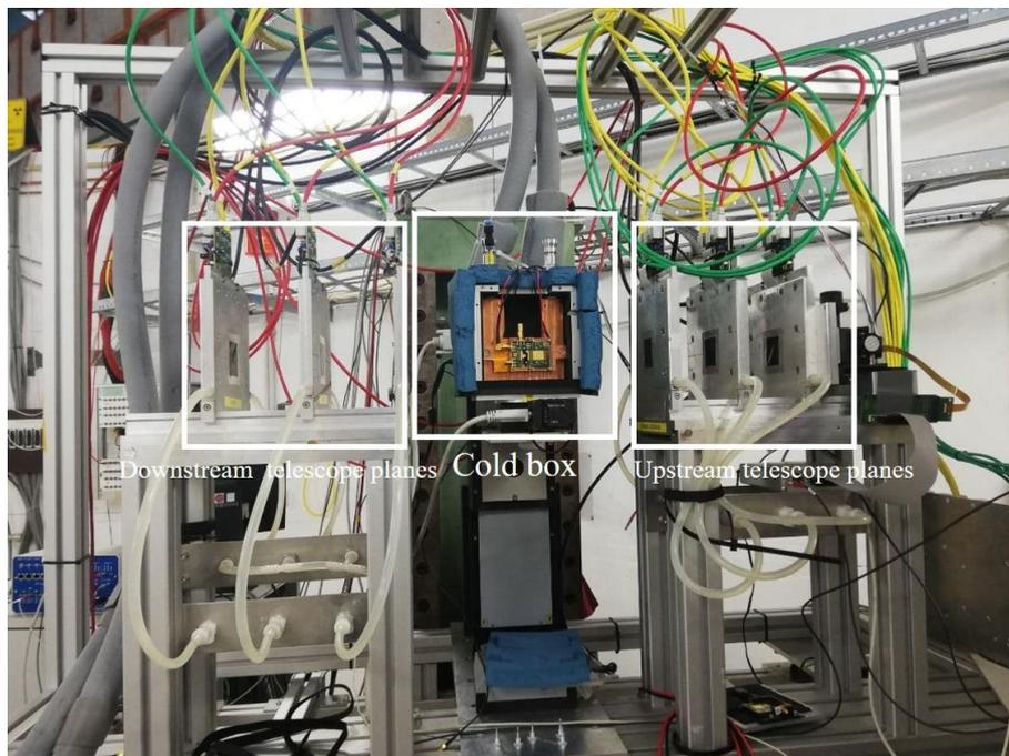
Figure 3.13: Test-beam setup for edge-on measurements with diodes.
